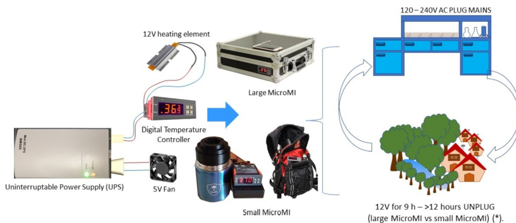
Fig. 1. The concept of MicroMI design (*) When unplugging from external electrical supply, the MicroMI with 12 V UPS maintains temperature from 9 to 12 h, depending on incubator size, external ambient temperature, and UPS battery capacity.
