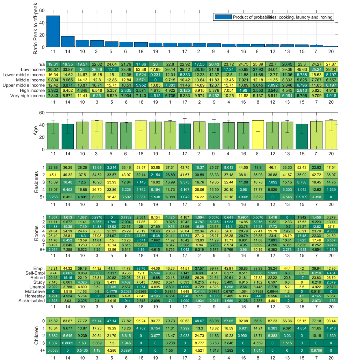
Figure 7: Comparison of peak to off-peak ratios by cluster and distribution of socio-demographic parameters for cluster composition (income group, age, number of residents, number of rooms, employment status and number of children). Clusters and corresponding socio-demographic information in descending order of product of peak to off-peak ratios of energy intensive activities.
