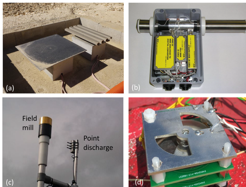
Figure 3. A selection of atmospheric electricity instruments. (a) Vertical current density sensor (GDACCS), using plate and corrugated electrodes, in the Negev desert. (b) Programmable Ion Mobility Spectrometer (PIMS) to determine electrical properties of air. (c) Electric field mill with sensing surfaces uppermost, and upward-pointing point discharge needle (not visible) with logarithmic current amplifier. (d) Miniature field mill with internal calibration electrodes.
