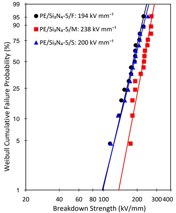
**Fig. 9** Weibull plots comparing DC breakdown strength of nanocomposites containing (a) 1 wt% of SiO<sub>2</sub>, (b) 5 wt% of SiO<sub>2</sub>, (c) 1 wt% of Si<sub>3</sub>N<sub>4</sub>, (d) 5 wt% of Si<sub>3</sub>N<sub>4</sub>, under fast, moderate, and slow crystallizations
