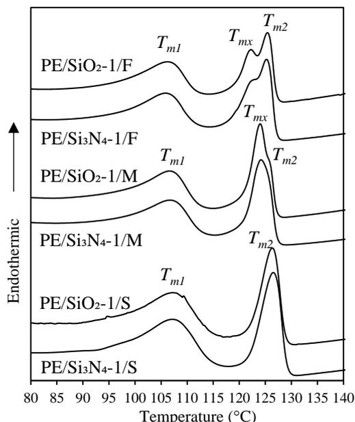
Fig. 2. Melting thermograms of nanocomposites containing 1 wt% of SiO<sub>2</sub> and Si<sub>3</sub>N<sub>4</sub>, when subjected to fast, moderate and slow crystallizations
