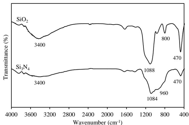
Fig. 4. FTIR spectra of  $\text{SiO}_2$  and  $\text{Si}_3\text{N}_4$  nanopowders
