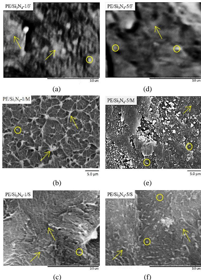
Fig. 7. Morphology of nanocomposites containing 1 wt% of  $\text{Si}_3\text{N}_4$  under (a) fast, (b) moderate, (c) slow crystallizations and nanocomposites containing 5 wt% of  $\text{Si}_3\text{N}_4$  under (d) fast, (e) moderate, (f) slow crystallizations
