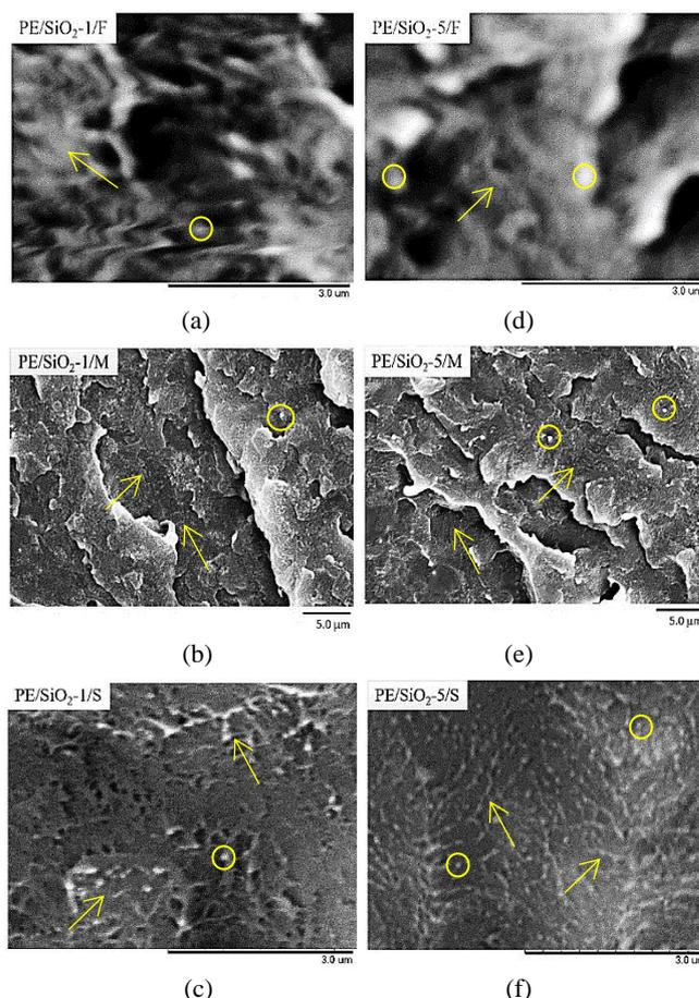
Fig. 6. Morphology of nanocomposites containing 1 wt% of  $\text{SiO}_2$  under (a) fast, (b) moderate, (c) slow crystallizations and nanocomposites containing 5 wt% of  $\text{SiO}_2$  under (d) fast, (e) moderate, (f) slow crystallizations
