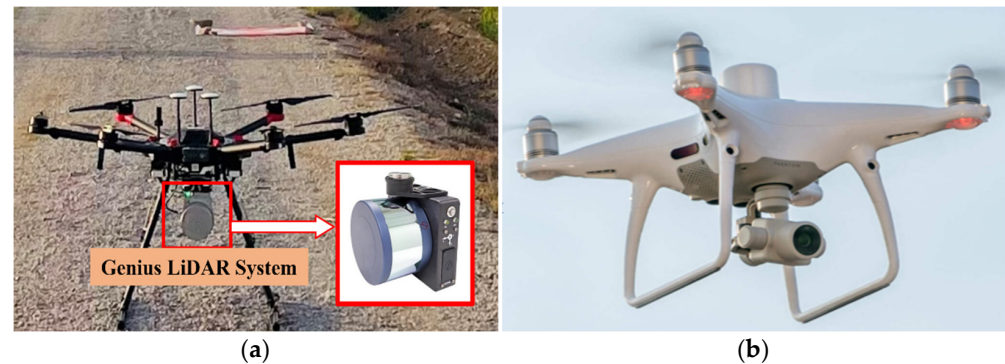
Figure 2. UAV platform: (a) DJI Matrice 600 Pro with Genius LiDAR system; (b) DJI Phantom 4 Pro.
