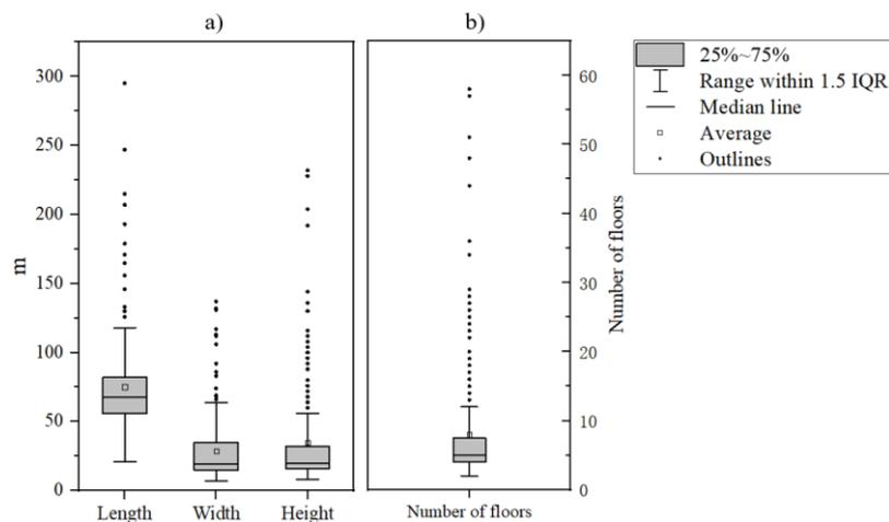
Figure 4: Main shape characteristics of typical office buildings
