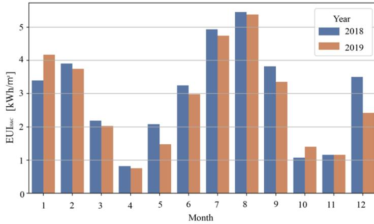
Figure 16: Monthly energy consumption of HVAC in 2018 and 2019
