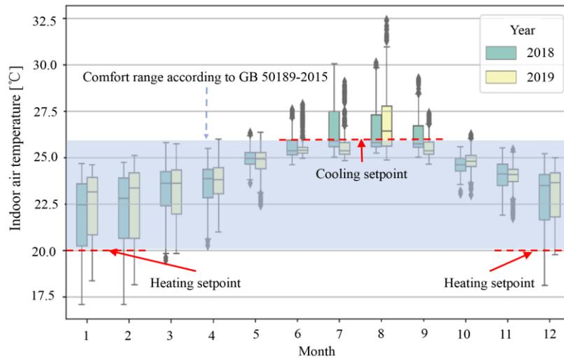
Figure 17: Monthly indoor air temperature during working hours
