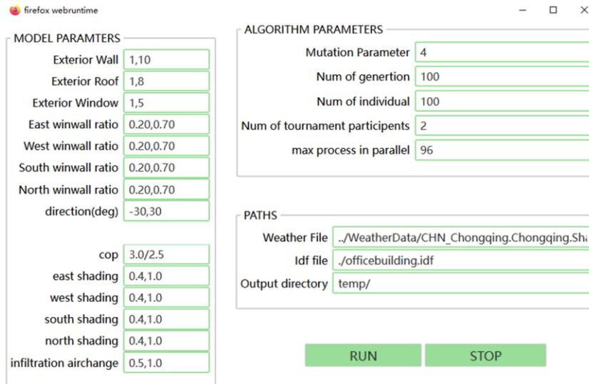
Figure 8: The input interface of the multi-objective model
