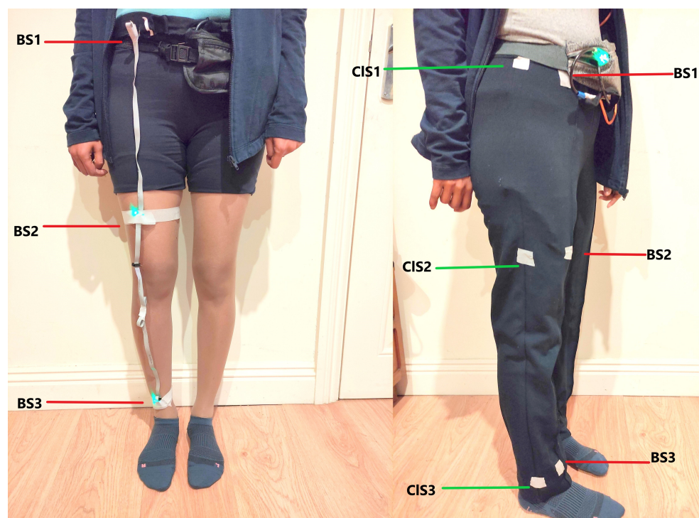
Figure 1. Sensor placement. On the body, there were three sensors on the frontal side of the body (BS1—waist, BS2—thigh, and BS3—lower-shank). On the clothing, there were three sensors along the lateral side of the lower body (CIS1—waist, CIS2—thigh and CIS3—lower-shank) in comparable positions to those on the body. Tape is used here to show the positions of the body-mounted and clothing-mounted sensors; however, in practice, neither was visible from the outside.
