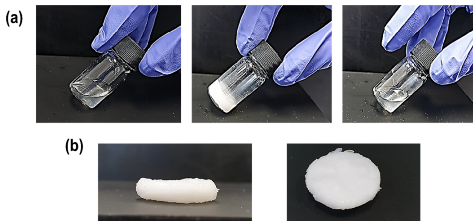
Figure 1. Solution–gel–solution transition of L-PEI cryogels. The solution is initially heated to 80 °C, forming a transparent solution. After freezing at –80 °C for 3 h and then thawing at room temperature, an opaque gel is obtained, which, on subsequent heating to 80 °C, returns to a transparent solution (a). Appearance of L-PEI cryogels (b).
