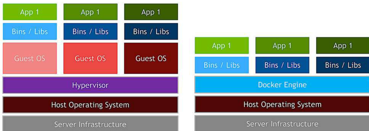
Figure 3: Operational background of classical virtual machines vs containers.
