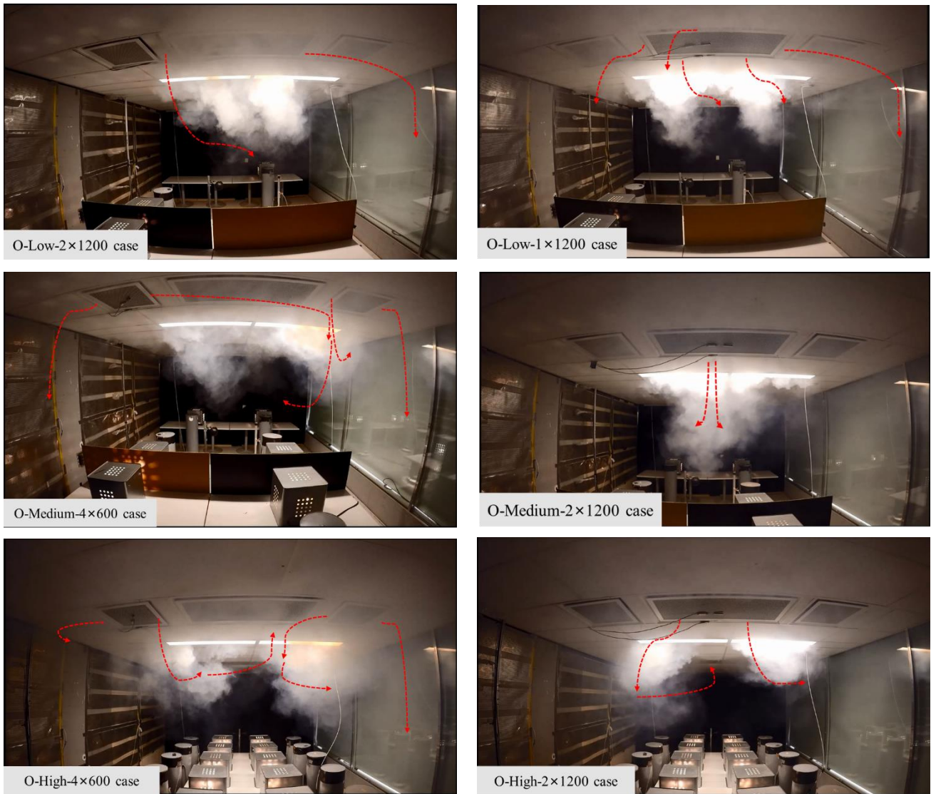
1 Fig. 5: The visualized airflow patterns under different heat gains and different chilled beam types. 2 (Note: Red arrows depict the direction of the supply air in those conditions.) 3
