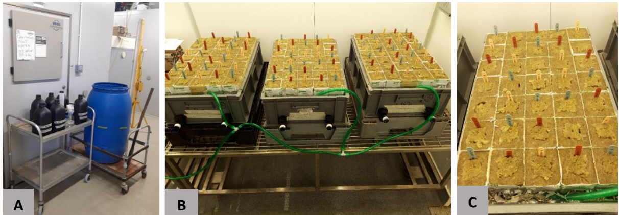
Figure 5.1. A) Fitotron plant growth chamber (WEISS Gallenkamp) set up for rice grain production (day and night temperatures 29 °C and 26 °C respectively, relative humidity 70%, PAR light intensity was 300–600 \mu\text{mol m}^{-2} \text{s}^{-1} at crop canopy, photoperiod was 10 h); B) supported hydroponic system; and C) tank ready for rice direct seeding in Rockwool cubes: each treatment (rice accession, priming treatment and salt treatment) had eight replicates, represented with the same labelling colour, and randomly distributed.
