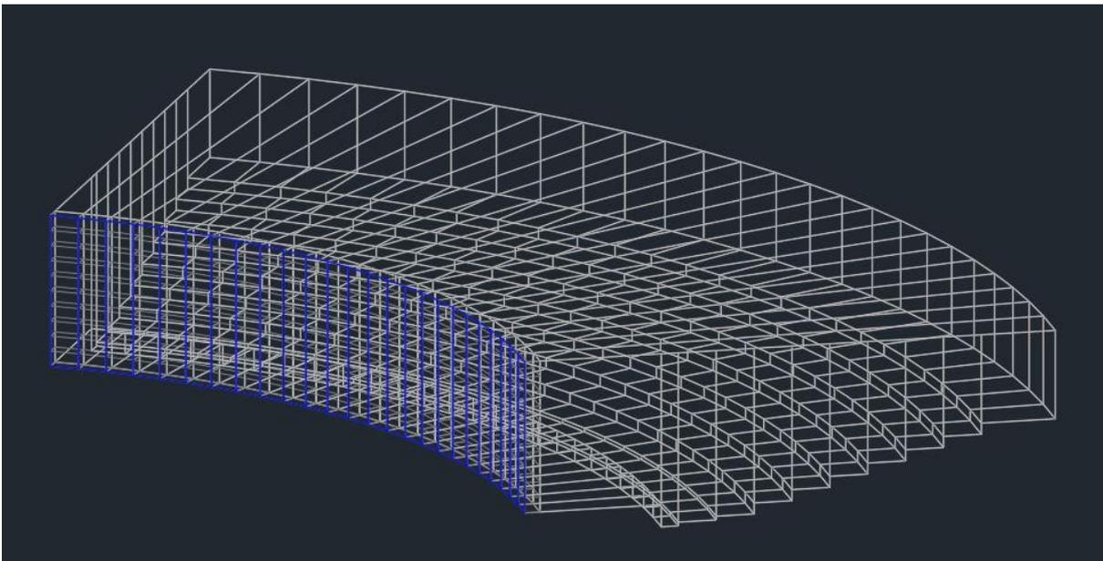
Figure 2: Mesh generation of the auditorium (white lines) and the DSF system (blue lines) – view from the south-east side.
