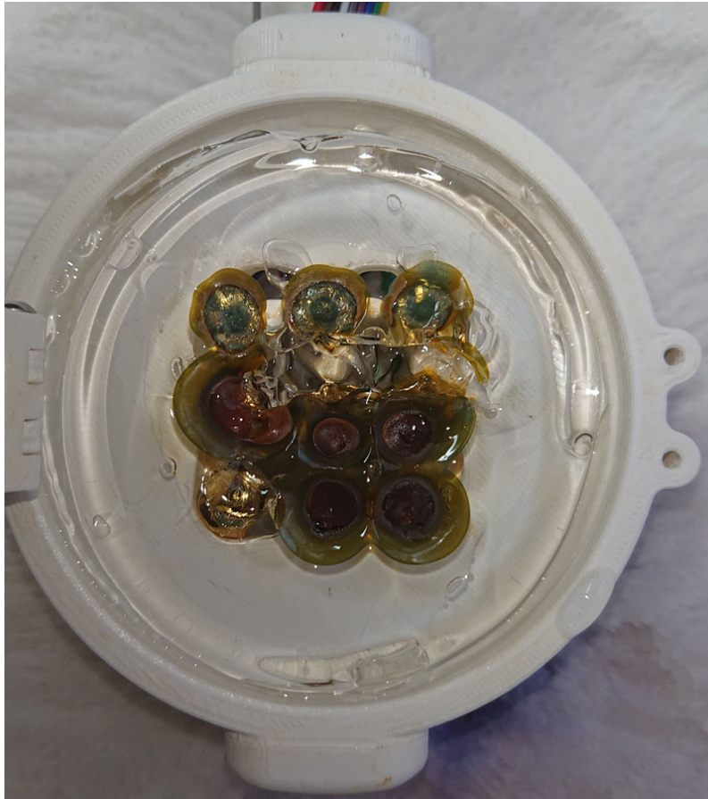
Figure A.14: At the point of deterioration the EAP gel forms a large hole in the centre as a result of the repeated electric stimulation breaking down the EAP gel structure. Once the hole has formed the sensing electrode pairs are separated from the stimulation electrode pairs and so the EAP gel can no longer perform in the Pong game. Further degradation can be seen in the green/brown staining caused by contact with the electrodes over time.
