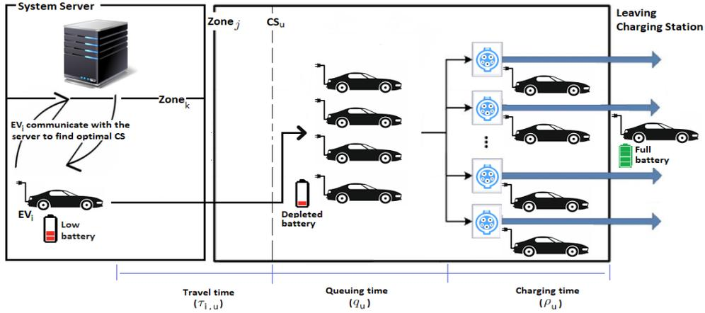
Fig. 4. Illustration of charging process completion time.
