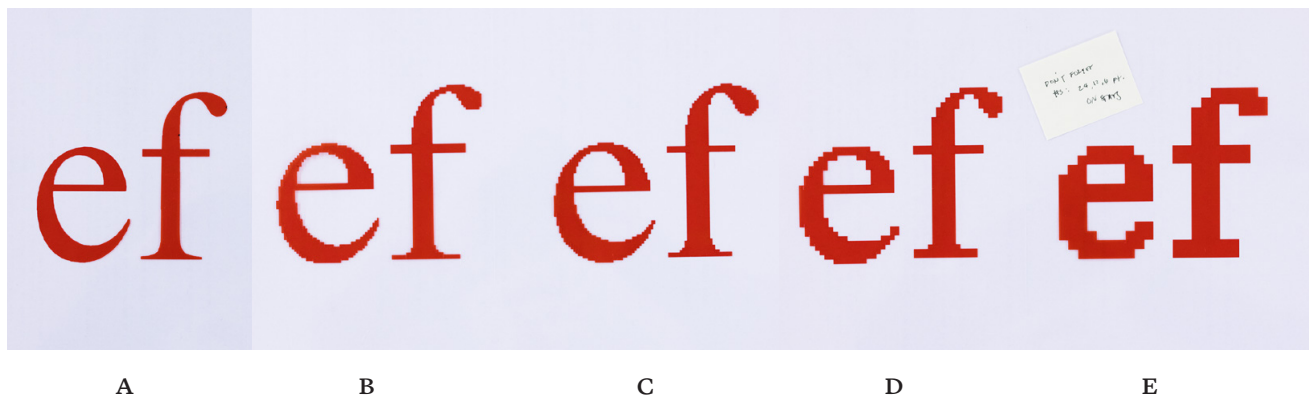
Fig. 4.110 Different sizes (pt) at resolutions (lpi) ranging between ‘high’ and ‘brick-laying’, adjusted in x-height for comparison: (A) 96 pt at 1000 lpi; (B) 12 pt at 1000 lpi; (C) 24 pt at 300 lpi; (D) 12 pt at 300 lpi; (E) 6 pt at 300 lpi. Plotter output, reproduced by Norman Posselt [CC, CSC 030, box 1, folder 5], overlapped here for comparison.
