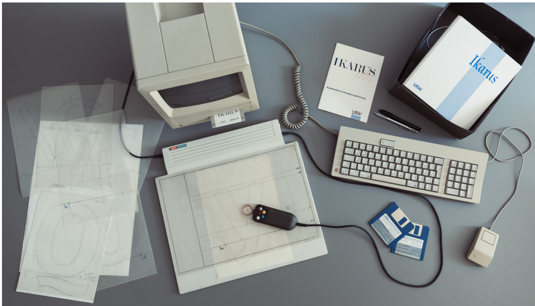
Fig. 5.18 Ikarus M type design system setup on an Apple Macintosh, equipped with Aristo tablet and digitizer, Apple keyboard and mouse and outline drawings of PT55 marked for digitization. Reconstructed from the personal collection of ES, photograph by Norman Posselt, 2017.
