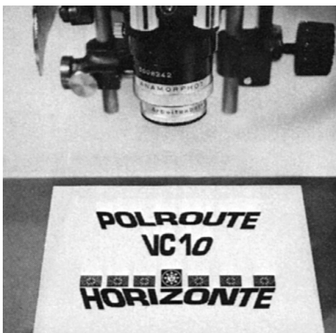
Fig. 5.28 Photographic lens distortion of Eurostile. Reproduced from the brochure Berthold Starsettograph , c. 1972.
