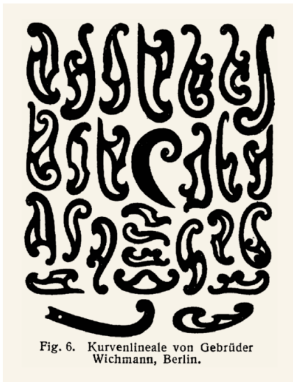
Fig. 4.37 Examples of 'Burmester-Schablonen' (manufactured by Wichmann Bros.), more commonly known as French curves, templates made from segments of clothoid spirals for drafting. Reproduced from Otto Luegner, Lexikon der gesamten Technik , 1904.
