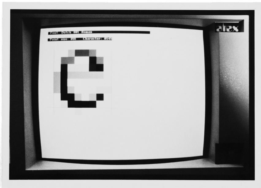
Fig. 4.114 Grey-scaling performed on an Atex monitor. Photographer unknown, reproduced by Norman Posselt [ibid.].
