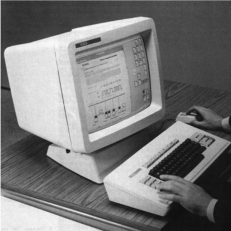
Fig. 4.89 Xerox 8010 'Star', the first commercial desktop workstation with a GUI of frames and icons. Reproduced from Seybold 1984, p. 366.
