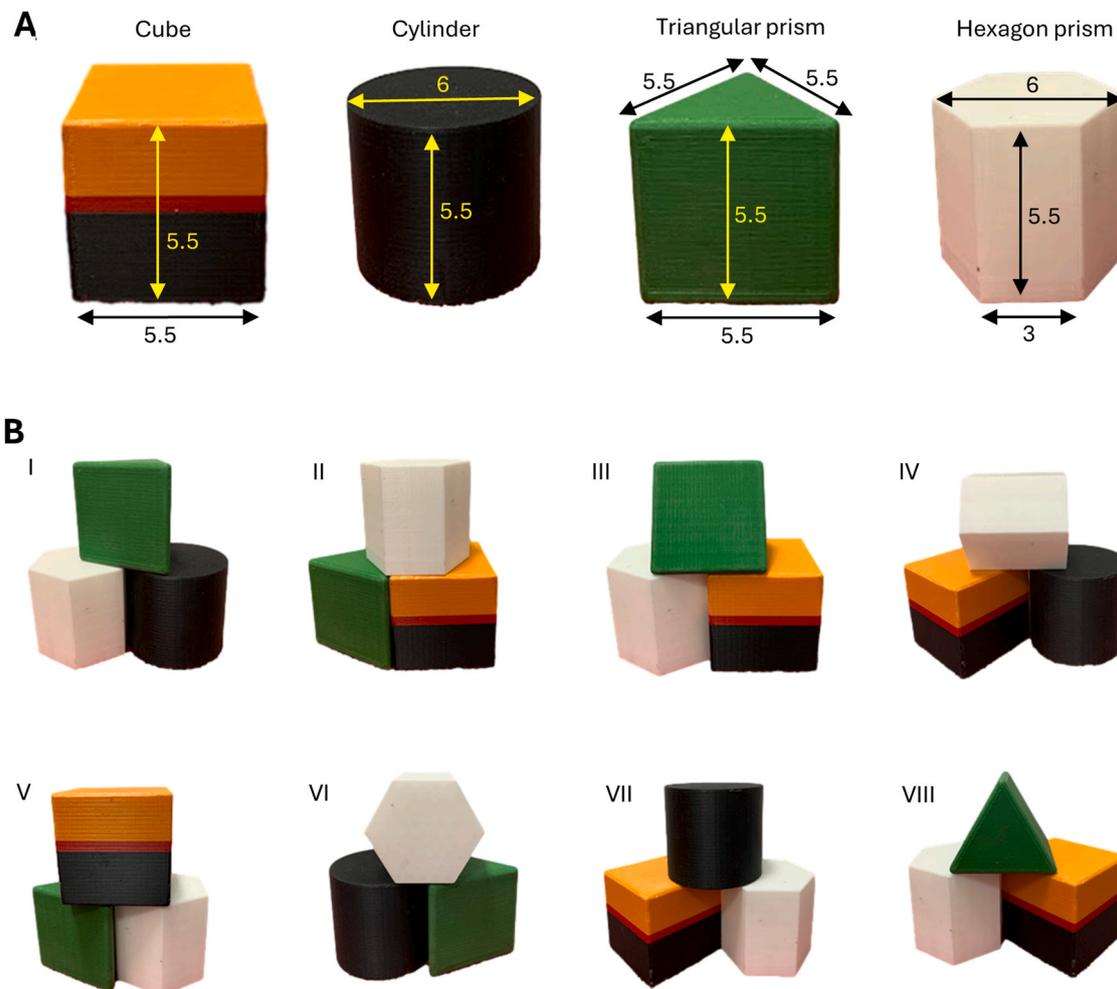
**Fig. 1.** Design of objects. (A) Photos and dimensions of four simple objects. (All dimensions are in cm.) (B) Photos of eight complex objects made from three simple objects. Note that the colour of each object is irrelevant to the task as all objects were covered in sandpaper during experiments.
