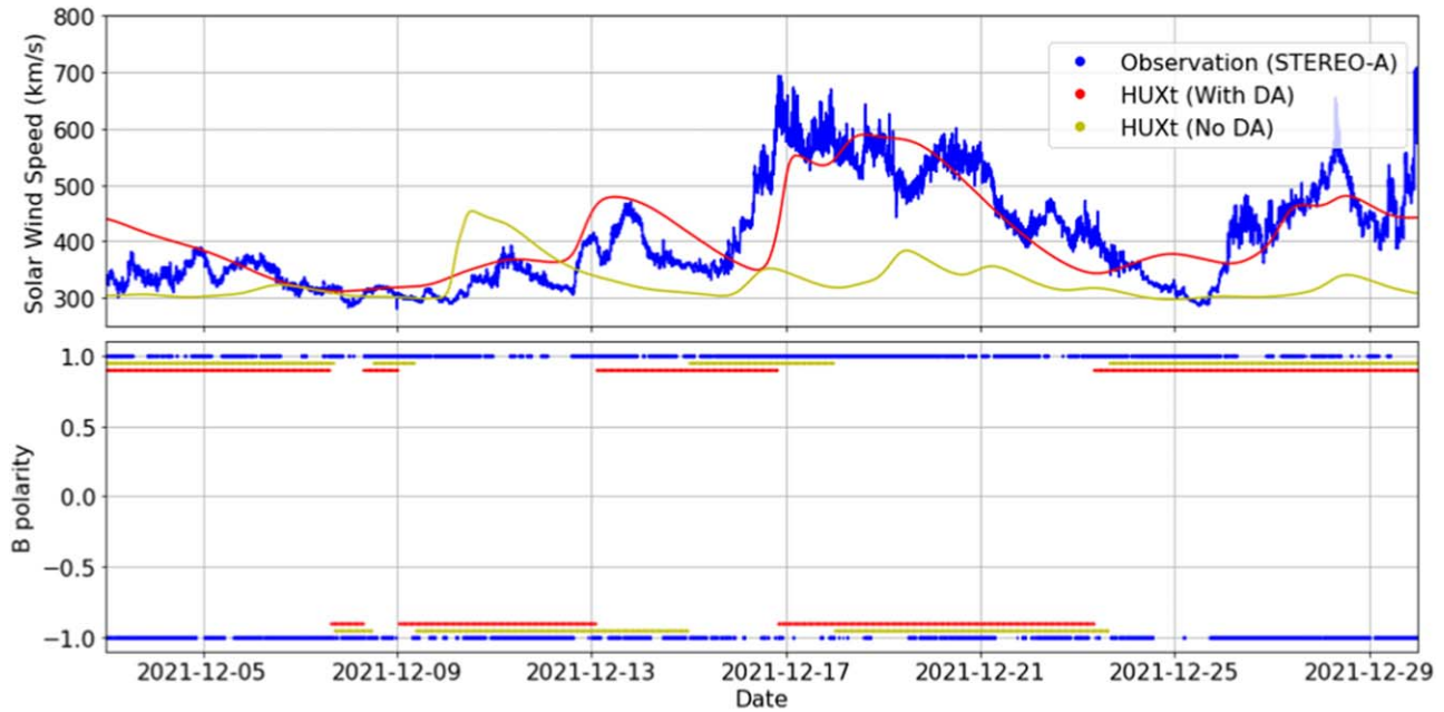
Figure 4. A time series of the solar wind speed (top) and magnetic field polarity (bottom) at STEREO-A for 2021 December. The MAS/HUXt model run (No Data-Assimilation) is shown in yellow and the MAS/BRaVDA/HUXt model run (Data-Assimilation) is shown in red, along with the observational data obtained from STEREO-A shown in blue over the same time period.
