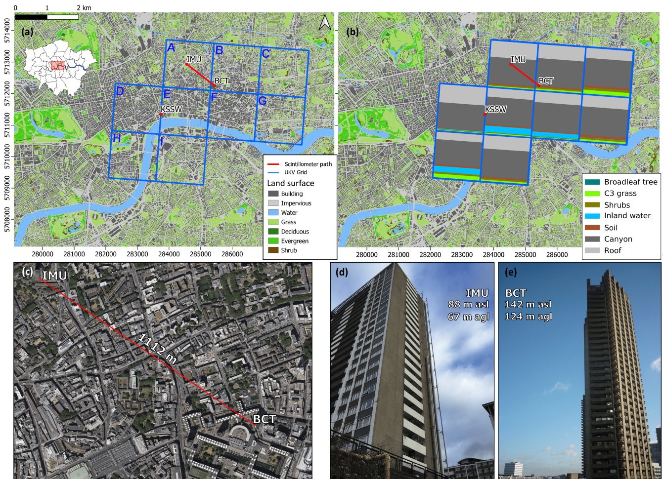
FIGURE 4 Study area with large-aperture scintillometry (LAS) path (red line), (a) land cover (based on Lindberg & Grimmond, 2011) shown in UTM zone 31 N (m) coordinates, and UKV grid boxes (blue, identified in text by labels A–I) and (inset) location in London (red rectangle); (b) UKV land cover proportions (Table SM.4); (c) aerial image (Bing Maps, 2021) of LAS path (red) region; and location of LAS (d) receiver (IMU) and transmitter (BCT). [Colour figure can be viewed at wileyonlinelibrary.com ]
