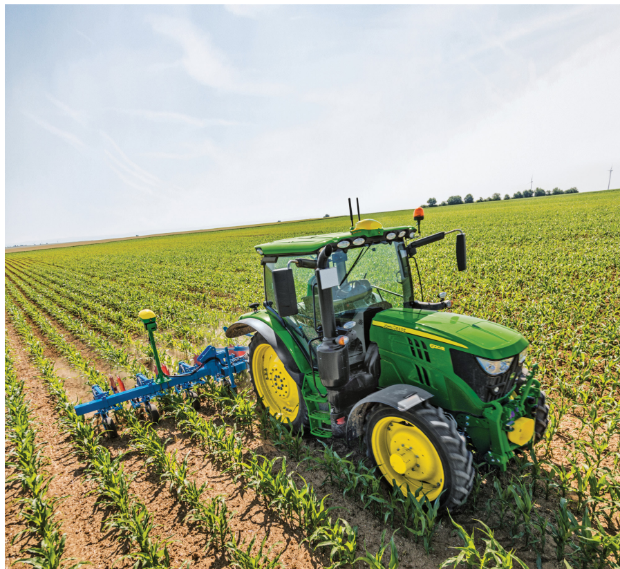
Precision inter-row mechanical weeding in a maize crop © John Deere.
