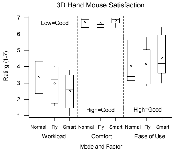
Figure 5. Hand mouse satisfaction and the effect of enhancement in 3D.
