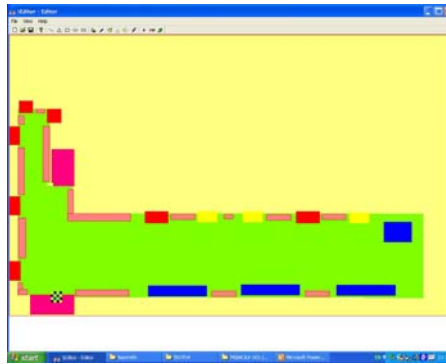
Figure 8. Haptic map of the environment appearing in Figures 6-7. The different colours are used to represent different haptic feedbacks.
