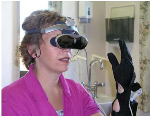
Figure 1. User wearing a head-mounted display (HMD) giving visual and a data glove that facilitates manual interaction in the virtual world.
