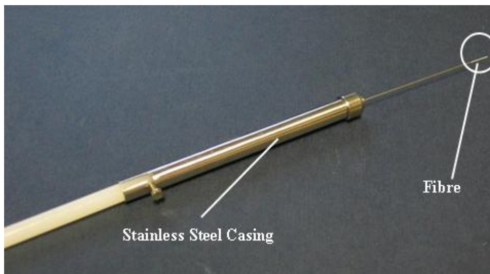
Figure 2. Diagram illustrating a plunged SPME showing its fibre
