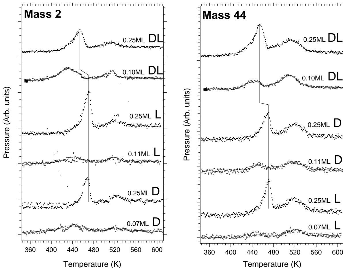
Figure 4: TPD spectra of saturated and lower coverage ( $\approx 0.1$  ML) chemisorbed layers of L, D and racemic (LD) serine. Left: H<sub>2</sub> partial pressure vs temperature; right: CO<sub>2</sub> partial pressure vs temperature.
