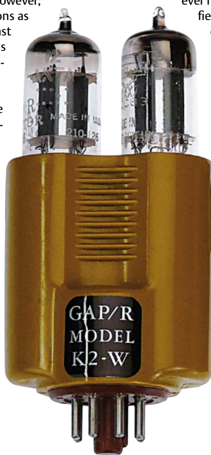
Figure 4. The Philbrick K2-W is generally considered the first commercial operational amplifier.
