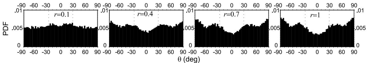
**Figure 12.** The histograms of the normalized crack length distribution against the angle around the compression direction,  $x$ , for varying  $r$  and a wind speed of  $10 \text{ m s}^{-1}$  under uniaxial compression. The same filtering as before is applied.
