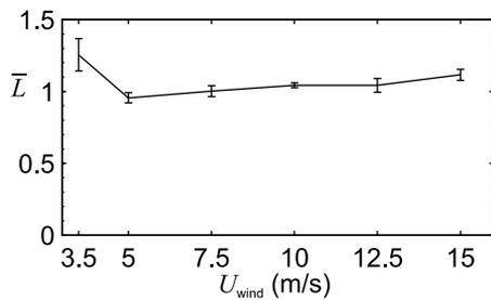
**Figure 9.** The normalized block size (square root of the block area divided by  $L_b^s$ ) for different wind speeds under uniaxial compression. The standard deviation is derived from mean block sizes for ten different ice field configurations. Blocks 10 times smaller than the average floe area are filtered out. The estimated block size  $L_b^s$  is 33, 27.6, 22.6, 19.5, 17.5, and 16 km for a wind speed of 3.5, 5, 7.5, 10, 12.5, and 15  $\text{m s}^{-1}$ , respectively.
