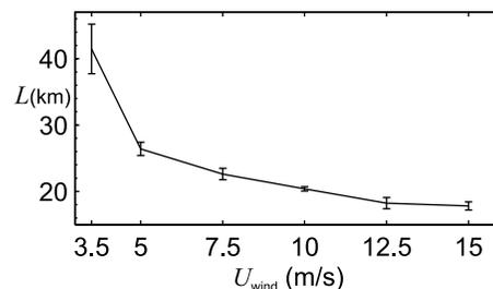
**Figure 5.** The normalized block size (square root of the block area) for different wind speeds under uniaxial compression. The standard deviation is derived from mean block size for 10 different ice field configurations. Blocks 10 times smaller than the average floe area are filtered out.
