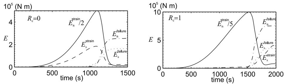
**Figure 19.** The stored elastic strain energy normal to the joints (solid line) and tangential to the joints (dashed line) versus time for a particular ice field configuration shown in Figures 3 and 14. The accumulated failure (elastic) energy normal to the joint (dot-dashed line) and tangential to the joints (dotted line) are also shown for comparison. (left) The uniaxial compression case ( $R_c = 0$ ). (right) The uniform convergence case ( $R_c = 1$ ) for  $U_{wind} = 5 \text{ m s}^{-1}$ .
