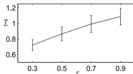
**Figure 18.** The block size normalized by  $L_b^s$  for varying  $r$  under uniform convergence ( $R_c = 1$ ). The standard deviation is derived from mean blocks sizes for nine different configurations. Blocks smaller than 10 times the average floe area are filtered out. The estimated block size due to shear rupture only,  $L_b^s$ , is 33.35, 37.89, 41.22, and 43.89 km for the relative tensile strength  $r = 0.3, 0.5, 0.7$ , and  $0.9$ , respectively ( $U_{wind} = 5 \text{ m s}^{-1}$ ).
