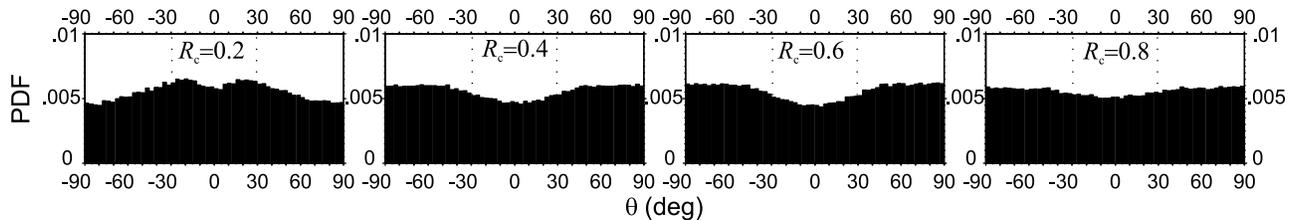
**Figure 15.** The histograms of the normalized crack length distribution against the angle around the compression direction,  $x$ , for varying confinement ratio  $R_c$ . The imposed wind speed is  $4 \text{ m s}^{-1}$  for  $R_c = 0.2$  and  $5.2 \text{ m s}^{-1}$  for the others. The case of  $R_c = 1$  is similar to that of  $R_c = 0.8$  with even higher uniformity in distribution. No filtering was applied. Run duration is 3000 s.
