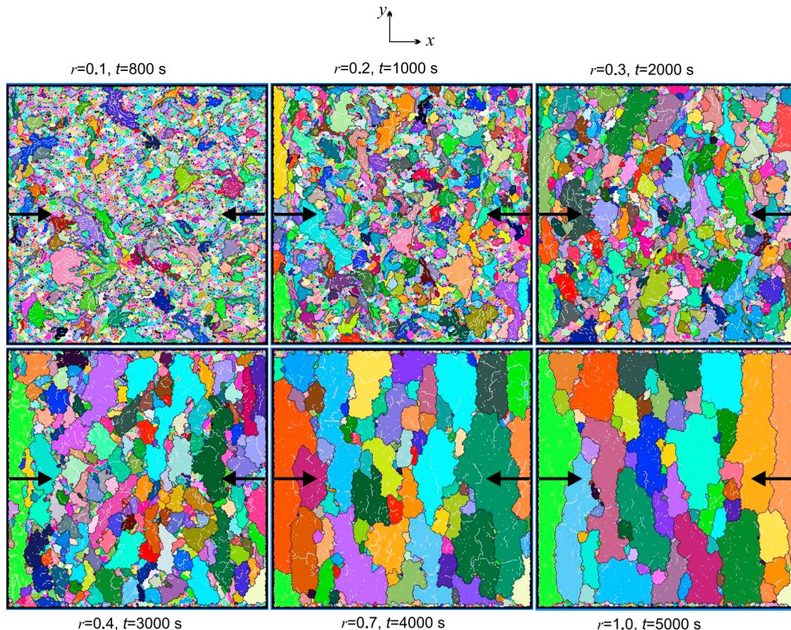
**Figure 10.** Ice cover for a varying relative tensile strength  $r$  and a wind speed of  $10 \text{ m s}^{-1}$  under uniaxial compression. Joints filtered out in the same way as before are shown in white. The black color shows joints delineating blocks used in our statistical analysis.
