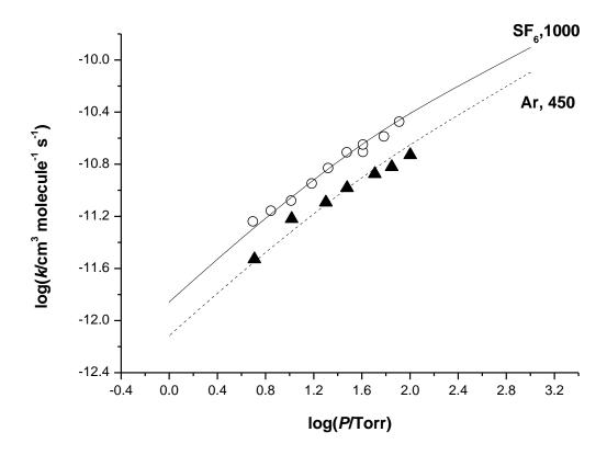
**Figure 9.** RRKM model (log  $(A/s^{-1}) = 16.0$ ) fits to the pressure dependence for SiH<sub>2</sub> + MeOH. Data points:  $\circ$ , SF<sub>6</sub>;  $\blacktriangle$ , Ar. Lines and step sizes indicated.
