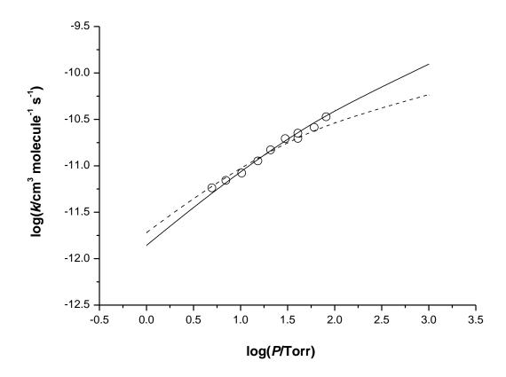
**Figure 8.** RRKM model fits to the pressure dependence for  $SiH_2 + MeOH$  (in  $SF_6$ ). Models: —,  $log (A/s^{-1}) = 16.0$ ; ----,  $log (A/s^{-1}) = 15.0$ )
