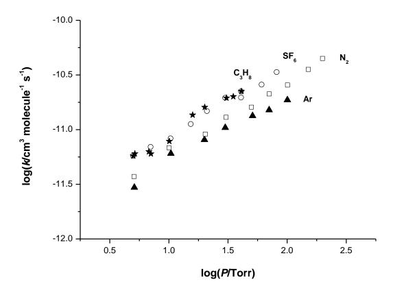
**Figure 2**. Pressure dependence of the second order rate constants for  $SiH_2 + MeOH$  at 297 K with different colliders, as indicated.
