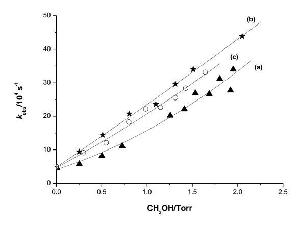
**Figure 1.** Second order rate plots for the reaction of  $SiH_2$  + MeOH at 297 K under various conditions:  $\blacktriangle$ , no buffer gas;  $\bigstar$ , 5 Torr total pressure (made up with  $SF_6$ );  $\circ$ , 2 Torr added  $SF_6$ . Lines are LSQ best fits: (a) and (c) quadratic; (b) linear.
