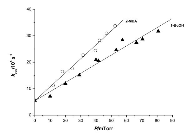
**Figure 4**. Second order plot for the reactions of  $SiH_2$  with 1-BuOH and 2-MBA at 10 Torr total pressure (added  $SF_6$ ) at 297 K.
