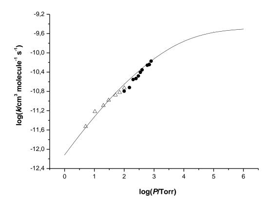
**Figure 12.** RRKM model (log  $(A/s^{-1}) = 16.0$ ) fit to the pressure dependence for SiH<sub>2</sub> + MeOH (in Ar). Experimental data:  $\triangle$ , this work;  $\bullet$ , reference 14.
