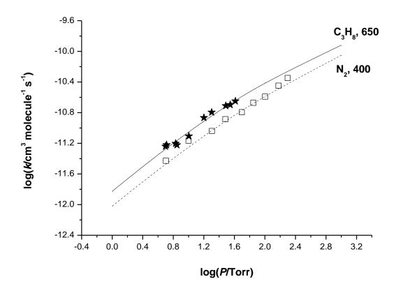
**Figure 10.** RRKM model (log  $(A/s^{-1}) = 16.0$ ) fits to the pressure dependence for SiH<sub>2</sub> + MeOH. Data points:  $\star$ , C<sub>3</sub>H<sub>8</sub>;  $\Box$ , N<sub>2</sub>. Lines and step sizes indicated.
