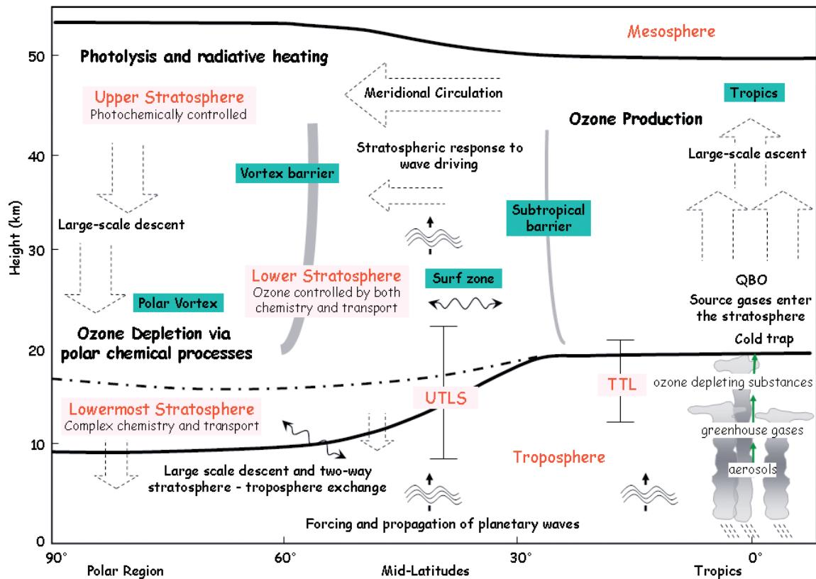
**FIG. 1. Schematic diagram of the principal regions and processes in the upper troposphere and lower stratosphere. Broad arrows denote diabatic circulation and wavy arrows denote transport along isentropic surfaces. The average position of the tropopause is shown by the lower thick-black line, the average position of the stratopause by the upper thick-black line, and the 380-K isentropic surface by the thick-black dot-dashed line. The vertical bars denote the range of the UTLS and TTL.**
