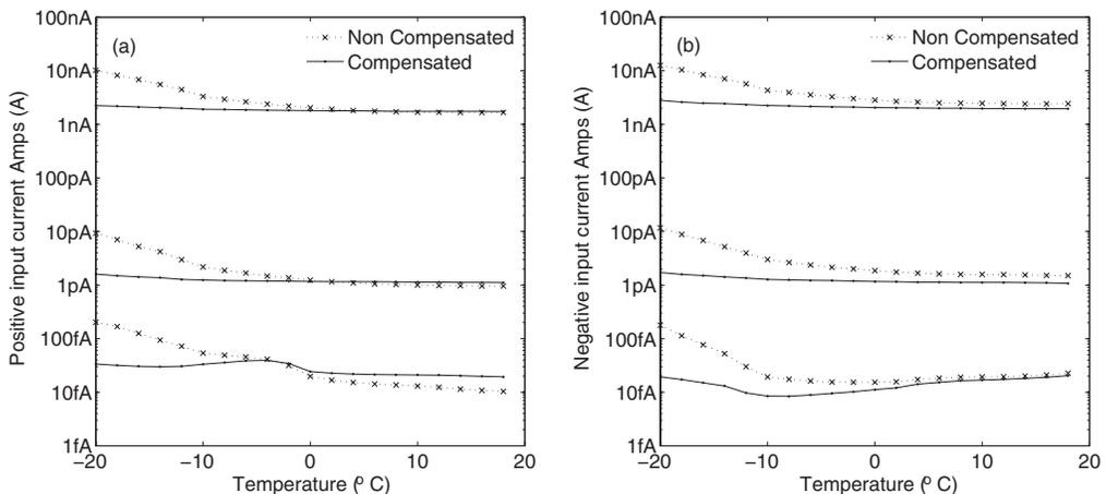
FIG. 3. Response of the PDC instrument to fixed currents (10 fA, 1 pA, and 1 nA) for uncompensated (dashed lines) and compensated (solid lines) outputs over the temperature range between  $-20$  and  $+20$  °C for (a) positive and (b) negative induced currents.
