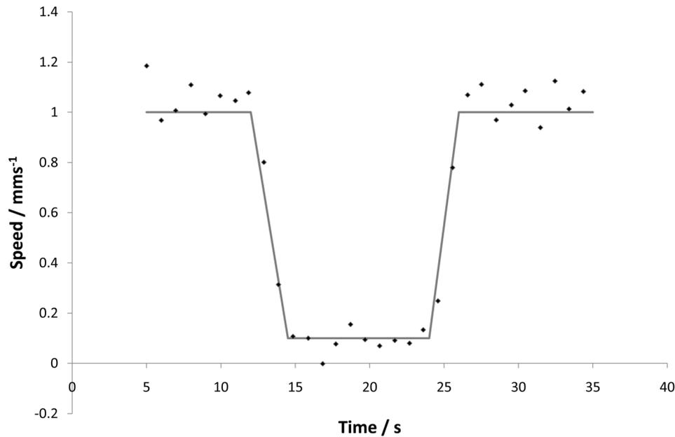
**Figure 8a.** A typical nonsteady state cycle, showing the pusher speed as a function of time. The diamonds show observations from a typical experimental cycle, while the solid line shows the numerical approximation used. Friction results for this cycle are shown in Figures 8b and 8c.
