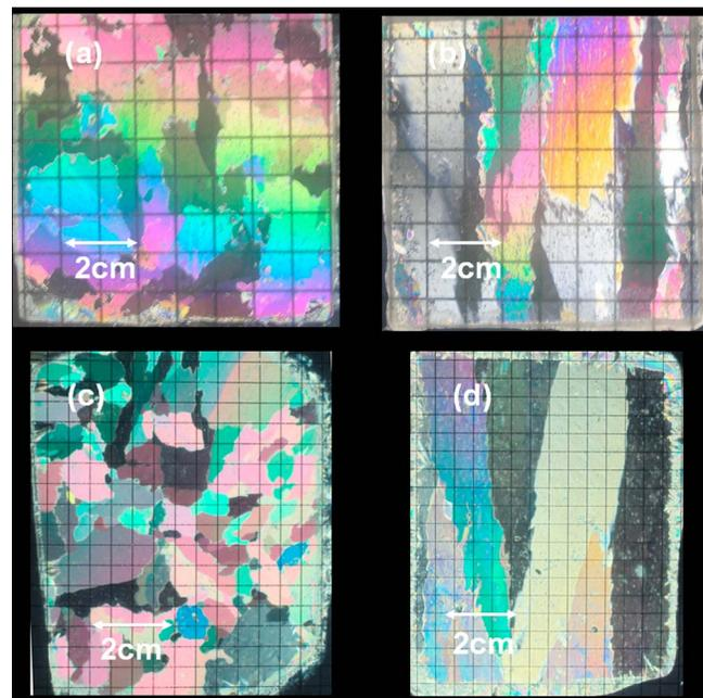
**Figure 3.** Thin sections of ice from (a) HSVA experiments,  $x$ - $y$  plane; (b) HSVA experiments,  $x$ - $z$  plane; (c) UCL experiments,  $x$ - $y$  plane; and (d) UCL experiments,  $x$ - $z$  plane. For the HSVA experiments the overlaid grid is marked out in centimeter squares and for the UCL experiments it is marked out in half centimeter squares.
