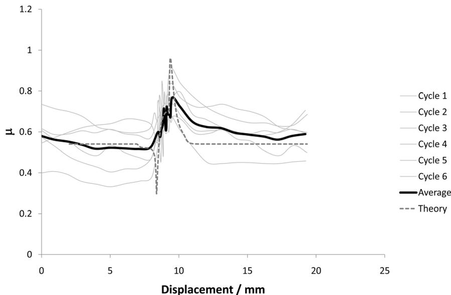
**Figure 8b.** Transient friction with varying speed (the speed cycle is shown in Figure 8a and the friction is plotted here as a function of displacement). The thin lines show results for six separate experiments, the bold line shows the average of these experiments, and the dashed line shows the prediction of our rate and state model for the given cycle.
