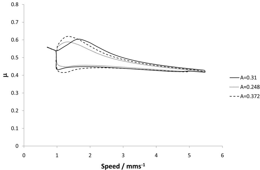
**Figure 10a.** Sensitivity test on the parameter  $A$ . The modeled data of Figure 8b (corresponding to the slip rate profile of Figure 8a) is replotted for  $A = 0.31$  (as in Figure 8b),  $A = 0.31 \times 0.8$ , and  $A = 0.31 \times 1.2$ .
