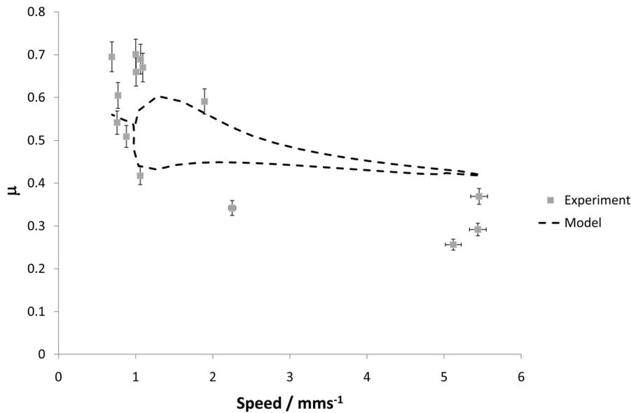
**Figure 9b.** Transient friction with varying speed (the speed cycle is shown in Figure 8a and the friction is plotted here as a function of displacement). The dashed line shows our numerical model, while the squares indicate experimental values, with vertical error bars representing uncertainty in the side load measurement.
