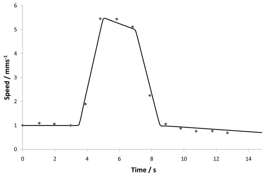
**Figure 9a.** A typical nonsteady state cycle, showing the pusher speed as a function of time. The diamonds show observations from a typical experimental cycle, while the solid line shows the numerical approximation used. Friction results for this cycle are shown in Figure 8b.
