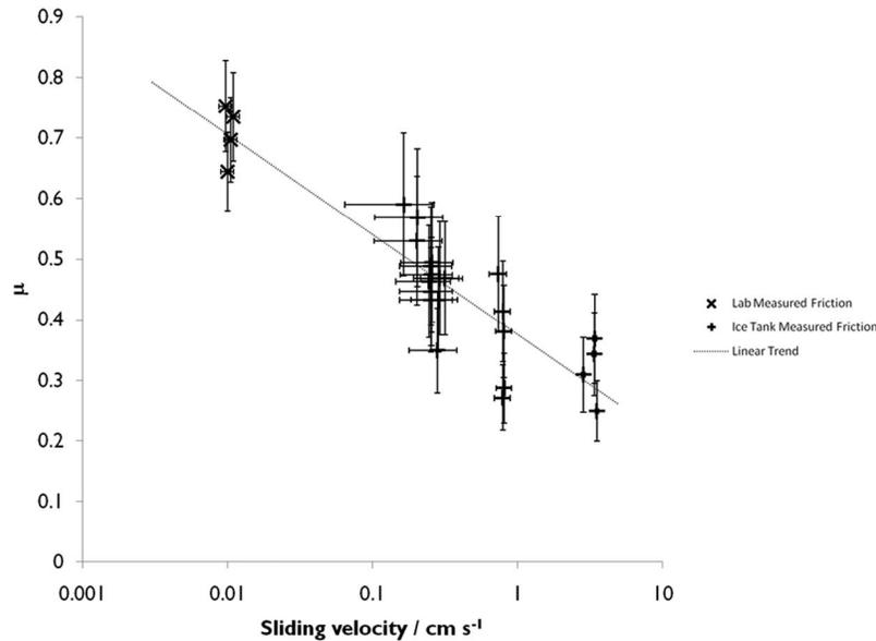
**Figure 5.** Experimentally determined rate dependence of sea ice friction. The crosses, at a sliding speed around  $0.1 \text{ mm s}^{-1}$ , are from laboratory experiments. The pluses, at higher speeds, are from ice tank experiments. The horizontal error bars represent variations in the pusher speed due to stick-slip behavior, while the vertical error bars represent variations in the normal load.
