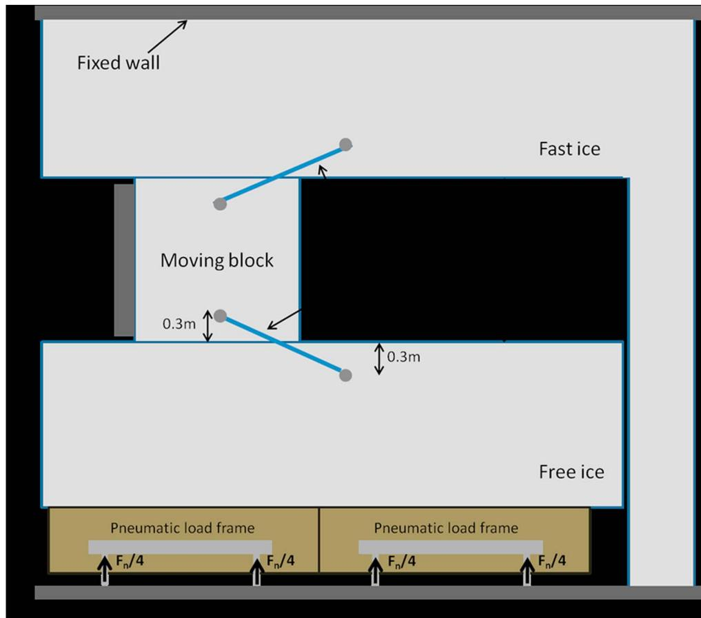
**Figure 4.** Schematic of ice tank experiments. The moving central ice block has dimensions  $2\text{ m} \times 2\text{ m} \times 0.25\text{ m}$ .
