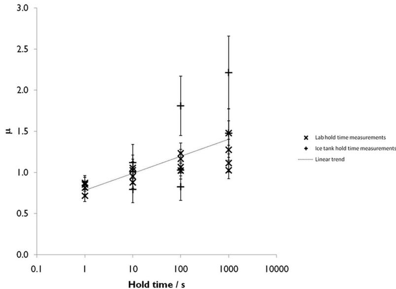
**Figure 6.** Experimental determination of the effects of static contact on the friction spike on resumption of motion. Crosses show laboratory data, while pluses show ice tank data. The dotted line shows a LMS linear fit to the data.
