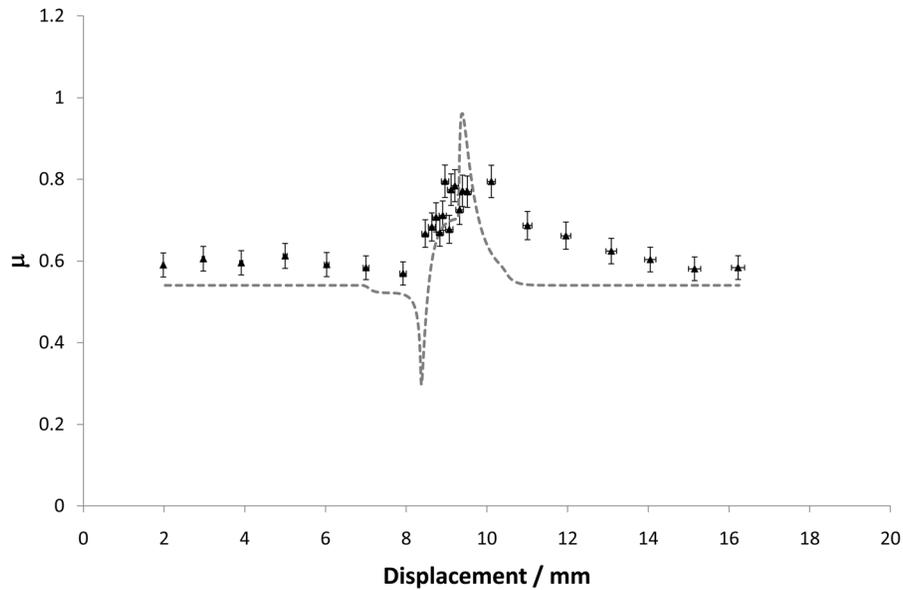
**Figure 8c.** Transient friction with varying speed (the speed cycle is shown in Figure 8a and the friction is plotted here as a function of displacement). The dashed line shows our numerical model, while the triangles indicate experimental values, with vertical error bars representing uncertainty in the side load measurement.
