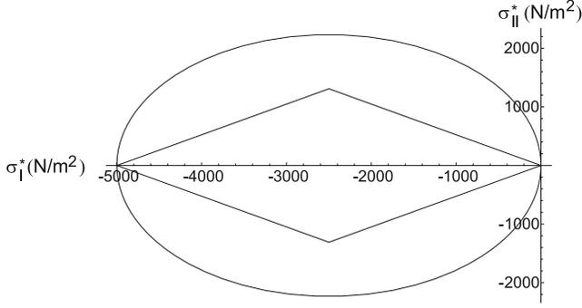
**Figure 4.** Yield curves in stress invariant space for two orientations of the square floes relative to the principal axes of the continuum-scale strain-rate ( $\beta^i = 0, \pi/4$ ), obtained using the elliptic material rheology. The yield curve at  $\beta^i = 0$  consists of four discrete points that are shown as joined lines.
