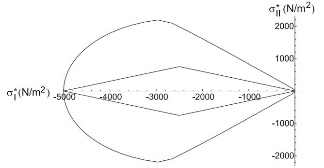
**Figure 8.** Yield curves in stress invariant space for two orientations of the square floes relative to the principal axes of the continuum-scale strain-rate ( $\beta^i = 0, \pi/4$ ), obtained using the modified elliptic material rheology. The yield curve at  $\beta^i = 0$  consists of four discrete points that are shown as joined lines.
