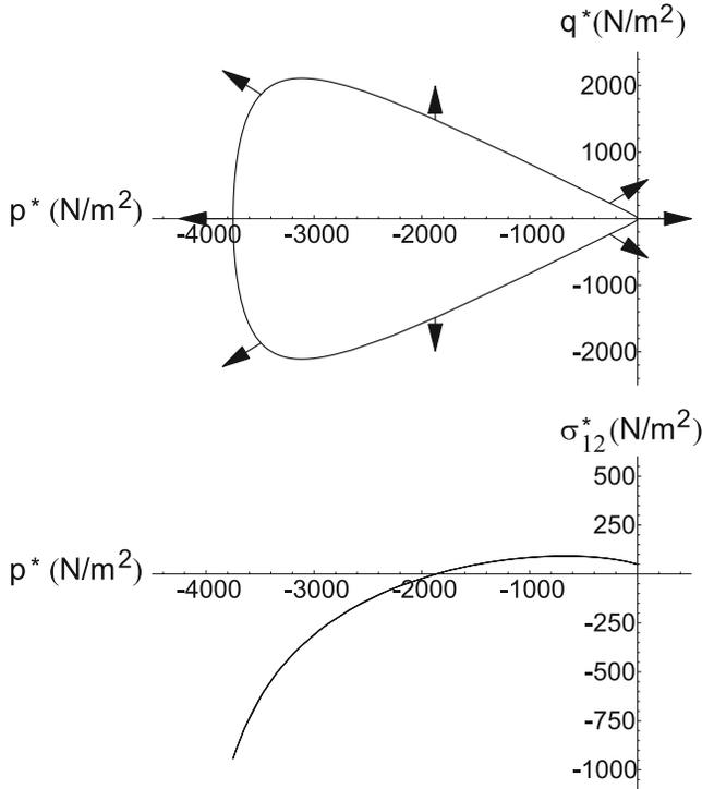
**Figure 10.** Yield curve projections onto  $p^* - q^*$  and  $p^* - \sigma_{12}^*$  planes for square geometry oriented at  $\pi/4$  to the principal axes of the continuum-scale strain-rate and linear material rheology in the anisotropic case (anisotropy fact  $\mu = 0.5$ ). The flow rule is also shown because the flow rule will be aligned with the  $p^* - q^*$  plane.
