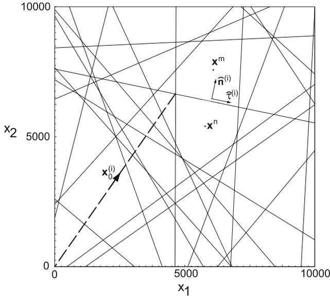
**Figure 1.** Definition diagram for two adjacent floes, with unit normal ( $\hat{\mathbf{n}}^i$ ) and tangent vectors ( $\hat{\boldsymbol{\tau}}^i$ ) for crack  $i$ , associated floe centroids with position vectors  $\mathbf{x}^m$  and  $\mathbf{x}^n$  ( $m < n$ ), and the position vector of the point on the crack from which arc-length is measured  $\mathbf{x}_0^i$ . The length of the  $i$ th crack is  $l^i$ .
