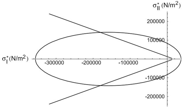
**Figure 3.** Yield curves at subcontinuum scale. Shown are the elliptic, linear, and modified-elliptic yield curves. The modified-elliptic yield curve consists of the linear yield curve to the right of the points of intersection with the ellipse, and the elliptical yield curve to the left of the intersection points.
