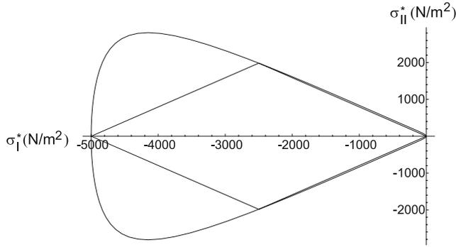
**Figure 6.** Yield curves in stress invariant space for two orientations of the square floes relative to the principal axes of the continuum-scale strain-rate ( $\beta^i = 0, \pi/4$ ), obtained using the linear material rheology. The yield curve at  $\beta^i = 0$  consists of four discrete points that are shown as joined lines.
