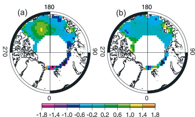
**Figure 5.** Modeled minus observed mean 1993–2001 winter thickness fields (m) for the model with (a)  $e = 2$ , and (b)  $e^2 = 0.5$ . Data are not available above 81.5°N [Laxon *et al.*, 2003].
