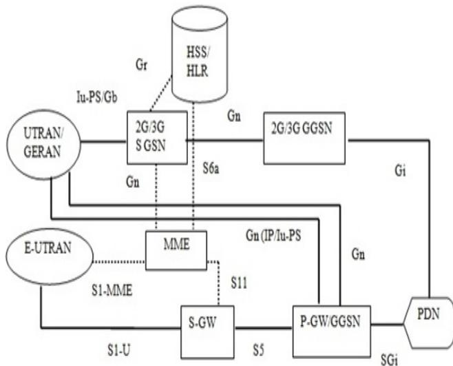
**Fig 4:** Architecture for E-UTRAN Interworking with GERAN/UTRAN (Pre-Release 8)-Source 3GPP
