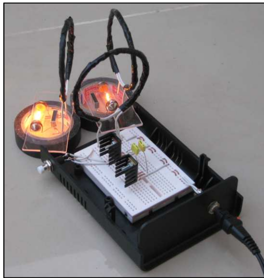
Fig.2.59. Operational oscillator powering multiple lamps.
