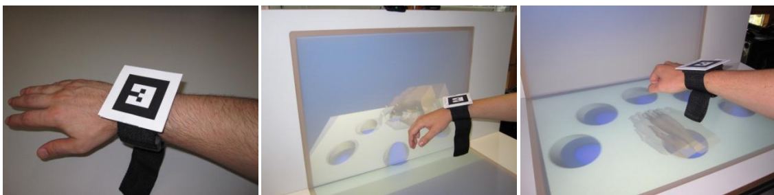
Figure 2. This simple arm shell is attached to the user's remaining arm stump using fiducial AR markers for tracking.
