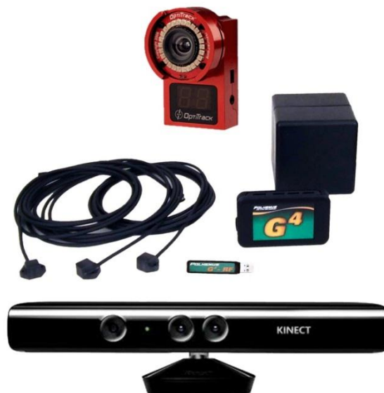
Tracking systems under study: optical; electromagnetic; and skeleton tracking.
