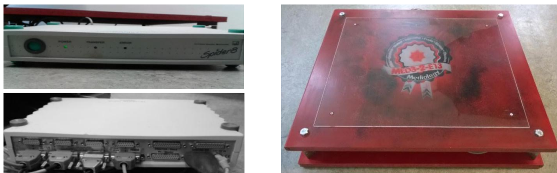
Figure 2. Spider 8 data logger (left) and balance board (right).
