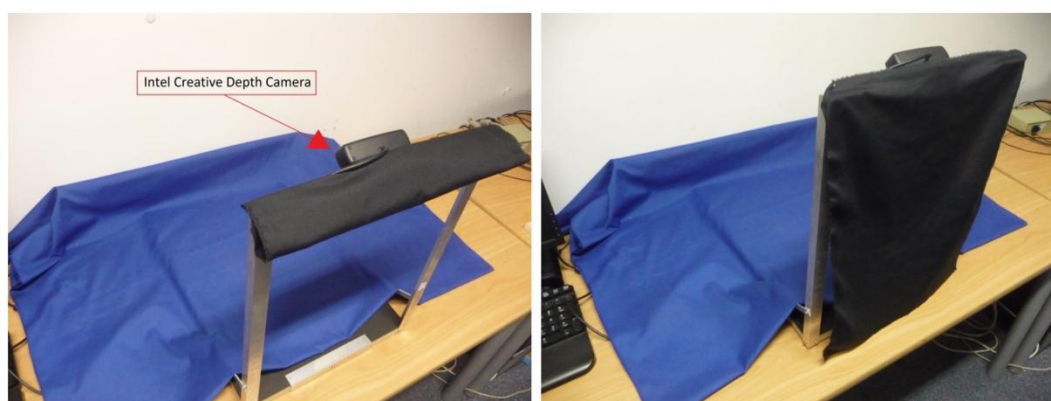
Figure 1. Metal Frame used to position the depth cam without curtain (left) and with the curtain to prevent the direct view of the hand during use (right).
