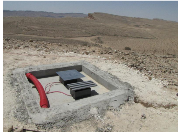
Figure 1. The GDACCS current density sensors at Mitzpe Ramon, Negev desert, Israel.
