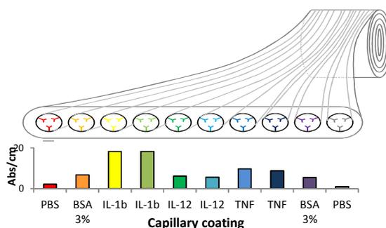
Femtomolar multiplex quantitation of human cytokines using disposable fluoropolymer microfluidic strips and a multisyringe aspirator capable of performing up to 80 tests using a flatbed scanner.
