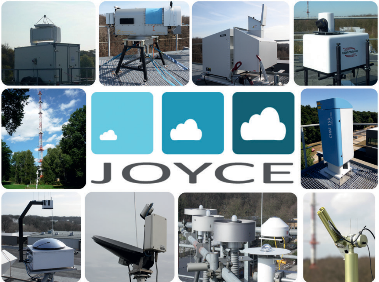
FIG. 2. Impression of selected JOYCE instruments. Clockwise from top left: cloud radar MIRA-36, microwave radiometer HATPRO, AERI, Doppler lidar Streamline, ceilometer CHM 15k, sun photometer CIMEL, radiation array, MRR, TSI, and 120-m meteorological tower.
