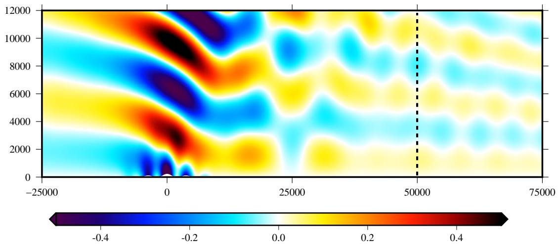
678 FIG. 6. Differences in potential temperature between the start and end of the gravity waves test on the BTF
