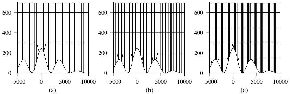
674 FIG. 5. Cut cell grids used for the gravity waves and thermal advection tests at (a)  $\Delta z = 300$  m, (b)  $\Delta z = 200$  m,
