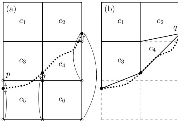
653 FIG. 2. Illustration of a cut cell grid (a) before, and (b) after construction. The terrain surface, denoted by a
