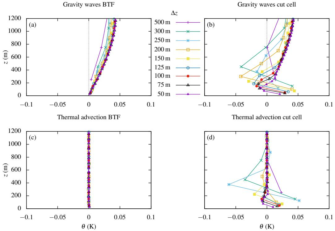
681 FIG. 7. Vertical profiles of potential temperature differences between the start and end of the gravity waves
