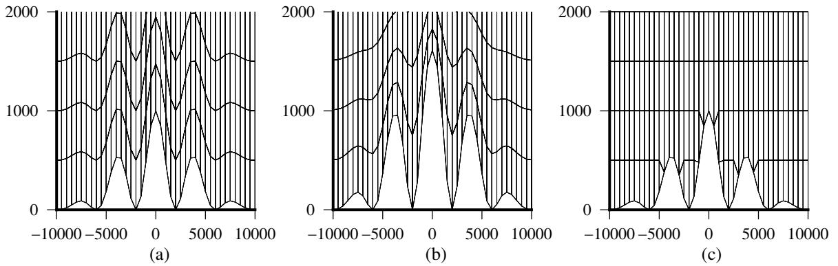
649 FIG. 1. Examples of (a) BTF, (b) SLEVE, and (c) a cut cell grid, showing cell edges in the lowest four layers.
