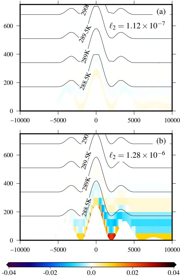
686 FIG. 8. Error in potential temperature (measured in K) in the thermal advection test at a resolution of  $\Delta z = 50$  m
