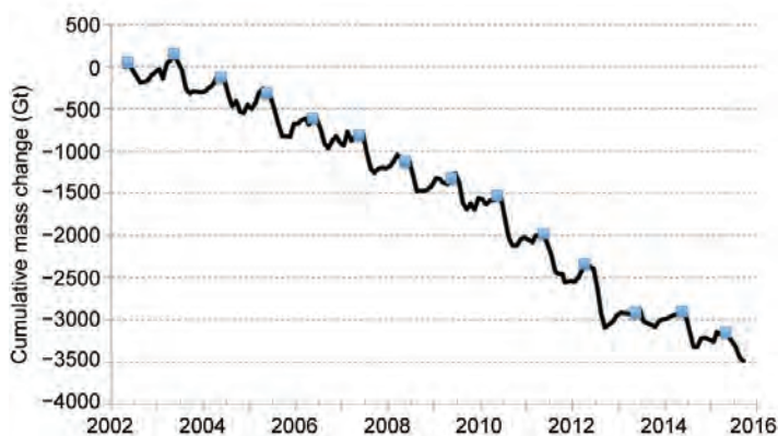
FIG. 5.10. Cumulative change in the total mass (Gt) of the Greenland Ice Sheet between Apr 2002 and Sep 2015 estimated from GRACE measurements. The square symbols denote Apr values for reference.
