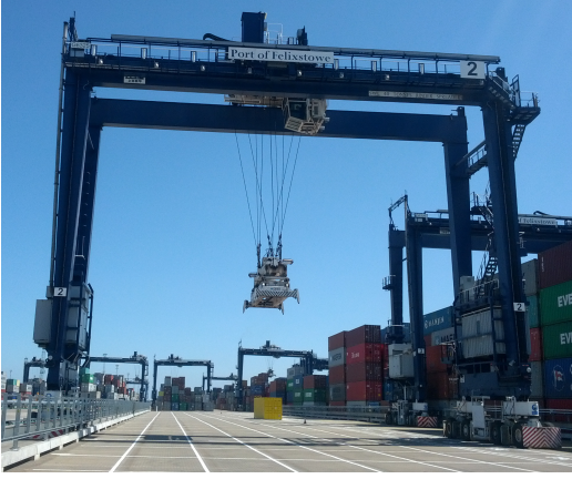
Fig. 2. Rubber-Tyred Gantry crane in use at the Port of Felixstowe.
