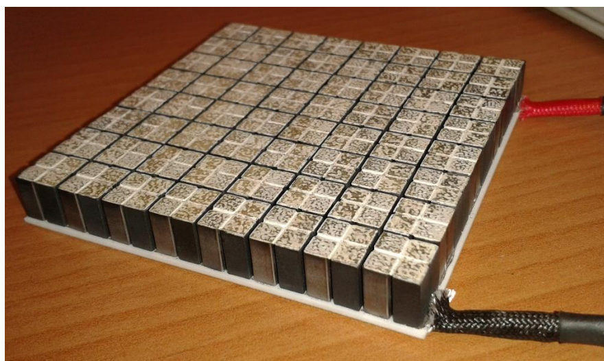
Figure 1.3 Picture of a thermoelectric module. (Taken at Crismat laboratories, Caen)
