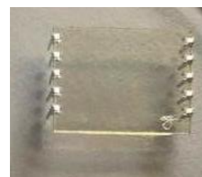
Figure 6.4a. Interdigitated ITO Substrates (Picture from Ossila: https://www.ossila.com/products/interdigitated-ito-ofet-substrates ). Figure 6.4b. Photo of a coated ITO cell used in this work
