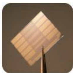
Figure 6.4a. Interdigitated ITO Substrates (Picture from Ossila: https://www.ossila.com/products/interdigitated-ito-ofet-substrates ). Figure 6.4b. Photo of a coated ITO cell used in this work
