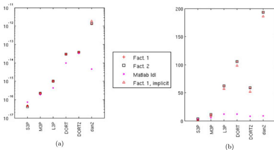
**FIGURE 5** Stability and sparsity results for  $\mathcal{F}$  matrices from a problem in fluid flow, as described in Section 4.3.2. (a) Backwards error (Equation 19), no iterative refinement. (b) Fill, as defined in Equation 20.
