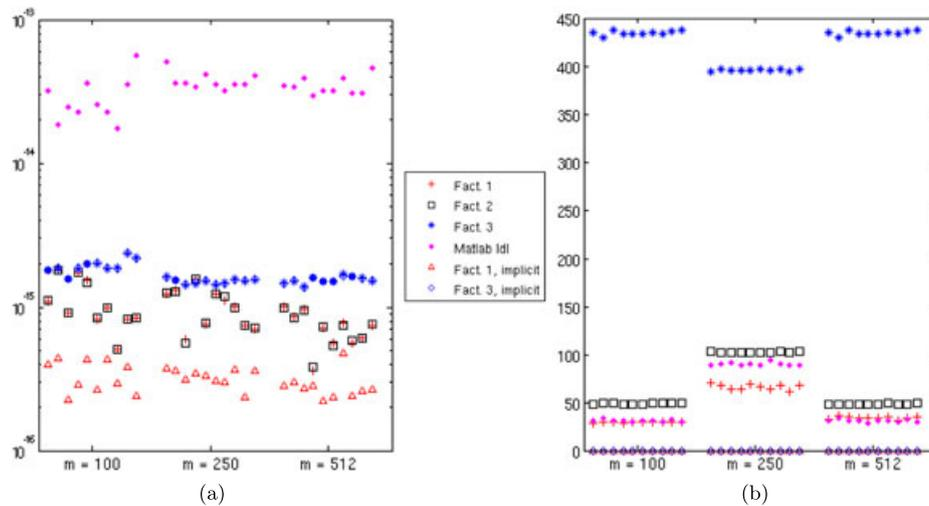
**FIGURE 4** Stability and sparsity results for the resistor network problem, as described in Section 4.3.1. (a) Backwards error (Equation 19), no iterative refinement. (b) Fill, as defined in Equation 20
