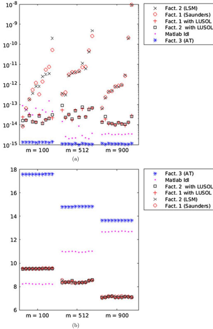
**FIGURE 1** Measures of stability and sparsity for various factorizations. The results given for 10 runs with small random matrices and are reported ordered by the worst performer. (a) Backwards error (Equation 19), without iterative refinement. The legend gives the order of performance, running from least accurate to most accurate (on average). (b) Fill, as defined in Equation 20. The legend gives the order of performance, running from least sparse to most sparse (on average)
