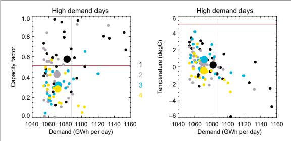
**Figure 6.** Daily electricity demand and GB mean wind power capacity factor (left) and mean 2 m temperature (right) during high demand days. Each day is coloured by its MSLP cluster number (see figure 5). The mean properties for each cluster are indicated by a large circle. The vertical grey line defines the lower boundary of the peak demand days and the horizontal red lines mark the winter average wind power capacity factor (left) and temperature (right).
