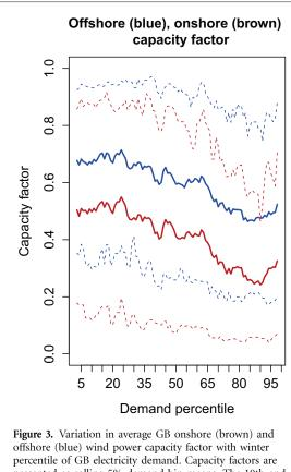
offshore (blue) wind power capacity factor with winter percentile of GB electricity demand. Capacity factors are presented as rolling 5% demand bin means. The 10th and 90th percentile capacity factors for each demand bin and each region are given (dashed).
