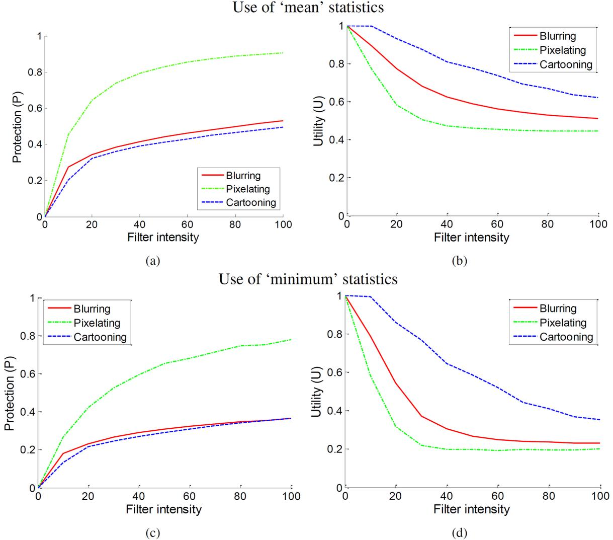
**Fig 4** Average protection score (a,c) and average utility score (b,d) obtained by blurring, pixelating and cartooning on all sequences of PEViD dataset for a variation of filter intensity. (a,b) P and U are computed using 'mean' statistics (i.e. Eq. 12, 17); (c,d) P and U are computed using 'minimum' statistics (i.e. Eq. 13, 18).
