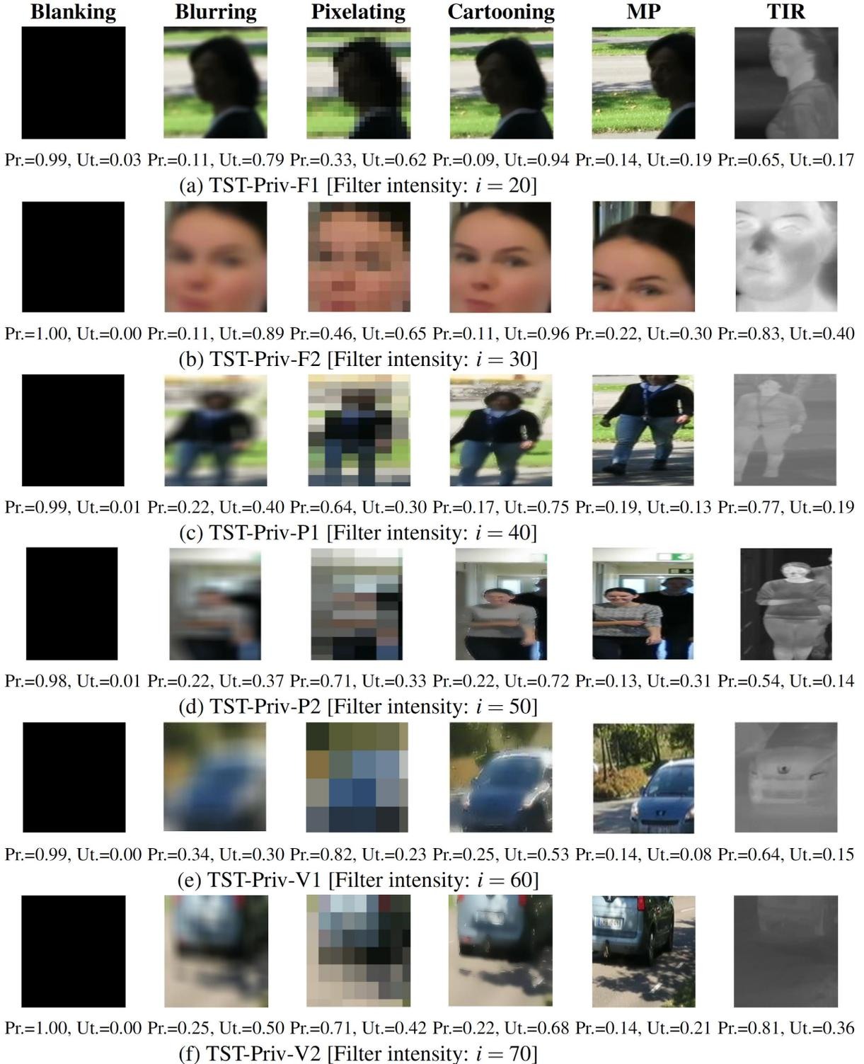
**Fig 3** Sample qualitative results for different privacy protection techniques applied on tracked patches with an increasing filter intensity ( $i = 20, 30, \dots, 70$ ). The corresponding protection (Pr.) and utility (Ut.) scores are also listed under each patch. Key. MP: motion perturbation; TIR: thermal infrared.
