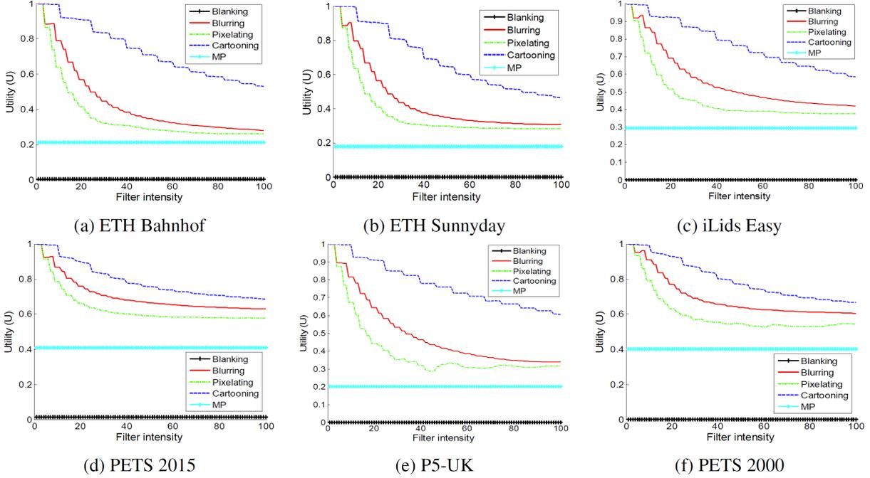
**Fig 11** Utility score (U) obtained by different privacy protection techniques for a variation of filter intensity on (a) ETH Bahnhof, (b) ETH Sunnyday, (c) iLids Easy, (d) PETS 2015, (e) P5-UK and (f) PETS 2000.
