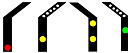
Figure 3. 5. These are examples of the additional stimuli that appear in experiment two. These are junction signals. When the angled bar above the signal is illuminated it means there is a change of track at the next trial. The change can be to the left or right. If the bar is not illuminated there is no change of track.
