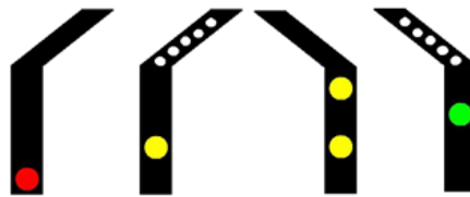
Figure 2. 2. These are examples of the junction signals. When the angled bar above the signal is illuminated it means there is a change of track at the next trial. The change is one step to the left or right.
