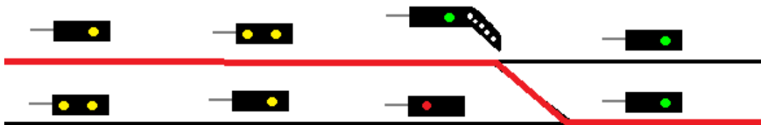
Figure 2. 12. This diagram illustrates a sequence of signals prior to and during a changing of track indicated by a junction signal. The red line marks the path that the subject follows, and the correct target stimulus are located immediately to the left of it.
