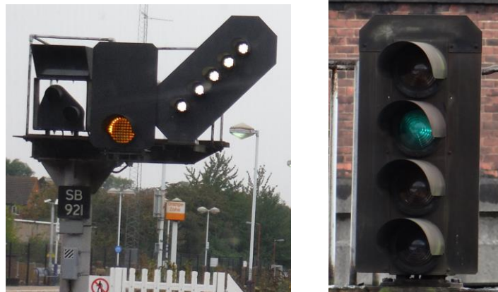
Figure 3. 1. The left photograph is of a junction signal used on the UK's national railway network. The yellow light means that the next signal is at red, meaning stop. The line of white lights indicate that the junction ahead is set for a right hand route. The right photograph is of a plain line (no junctions) signal that can display 4 possible aspects. This type is commonly found on busy sections of track.
