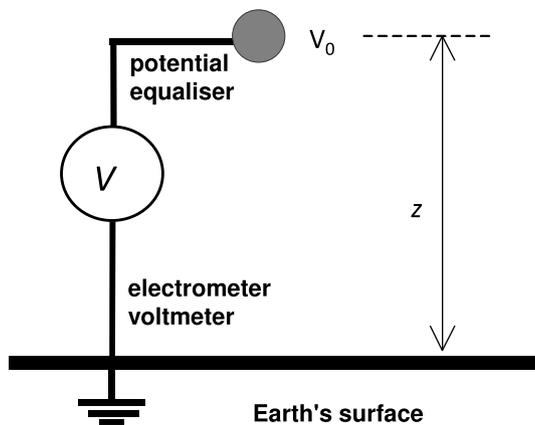
**Fig. A1.** Conceptual picture of the measurement of the vertical potential gradient (PG). A potential equaliser positioned at a height  $z$  comes into electrical equilibrium with the air around it, acquiring its potential  $V_0$ . The PG at height  $z$  is found as  $V_0/z$ .
