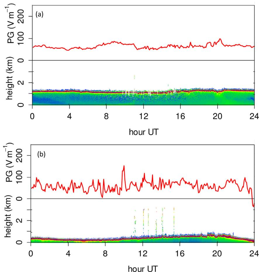
**Fig. 3.** Daily time series on cloudy days of ceilometer backscatter profile (lower half-panels) and PG (5 min means from 1 s samples) obtained at Reading University Atmospheric Observatory, for (a) 23rd March 2016, and (b) 3rd June 2016. The ceilometer colour scale is the same as in Fig. 1. (For interpretation of the references to colour in this figure legend, the reader is referred to the Web version of this article.)
