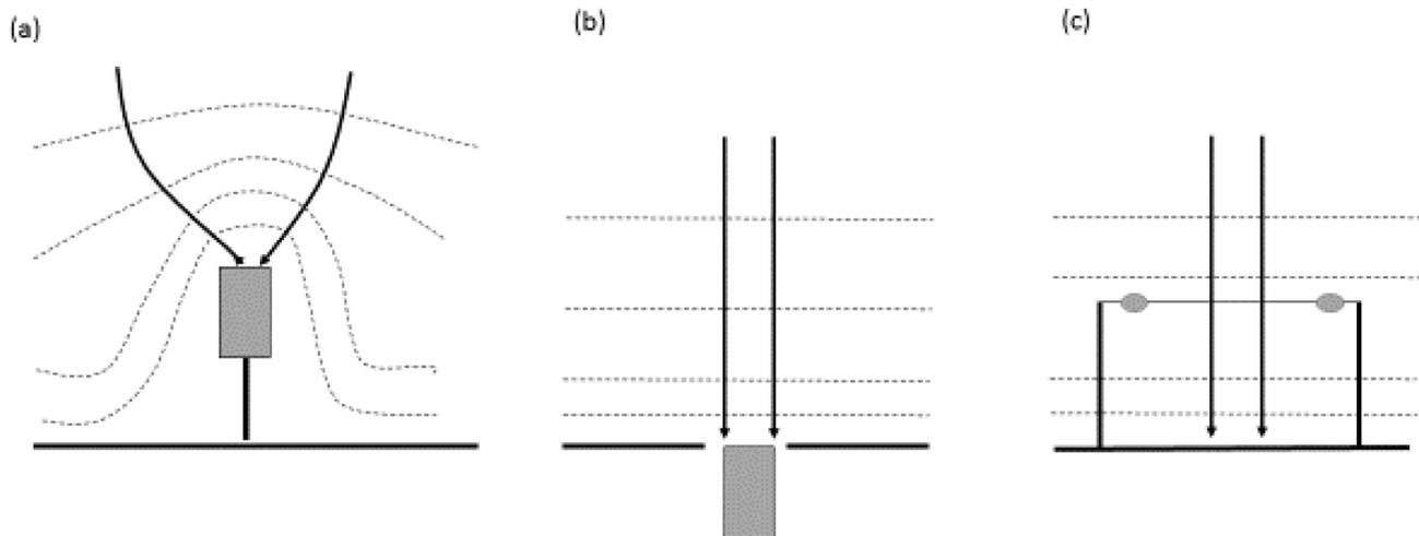
**Fig. A2.** (a) Effect of electric field distortion on a mast-mounted field meter. (b) Lessened effect of electric field line distortion by having the sensing surface of the field meter flush with the surface. (c) Use of a horizontal passive wire antenna to obtain the undistorted potential at a known height. (In each case, the dashed lines are equipotentials, and the solid lines are field lines).
