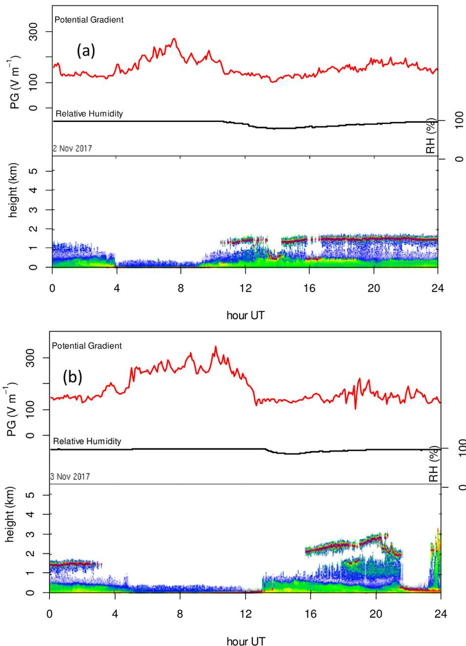
**Fig. 6.** Variations in Potential Gradient (PG) at Reading (upper panel) for two days with fog, (a) 2nd November 2017 and (b) 3rd November 2017. The relative humidity (RH) data from the site is also shown, and both this and the PG data are five minute average values from 1 s samples. The ceilometer colour scale is the same as in Fig. 1. (For interpretation of the references to colour in this figure legend, the reader is referred to the Web version of this article.)
