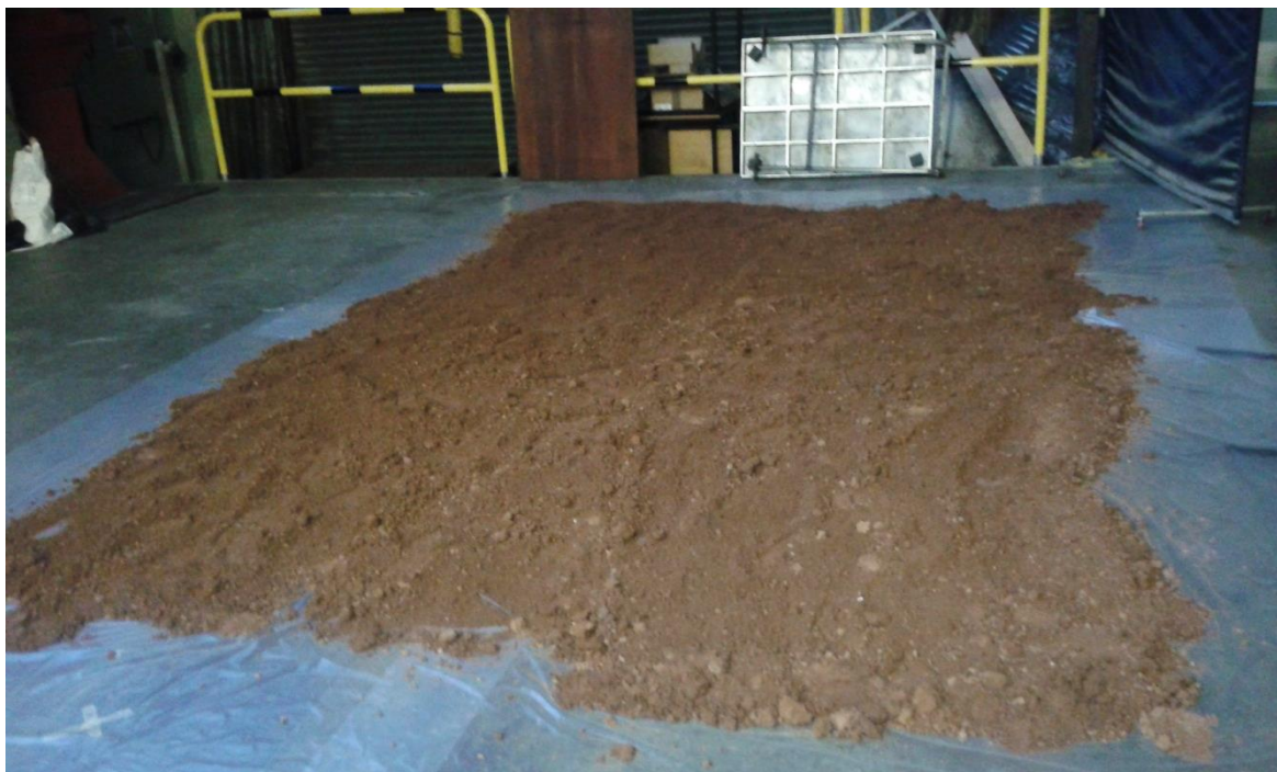
Figure 3-1: The British soil from Devon spread out on the laboratory floor in order to be dried out to reach an initial constant moisture content
