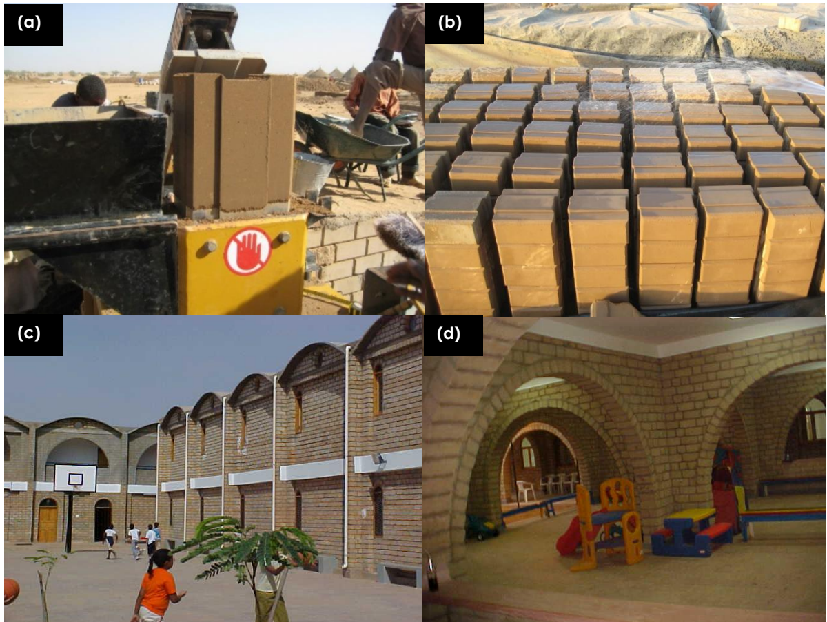
Figure 2-16: Compressed earth blocks technique, (a) how the block looks straight after production, (b) blocks stacked over each other after production, (c) Holm English Medium School in Khartoum, Sudan built completely using compressed earth blocks, (d) the interior of the school showing the exposed compressed earth blocks. Source: Author's collection
