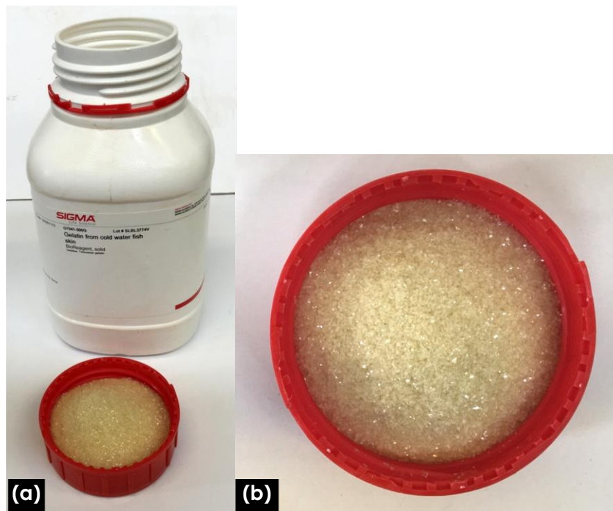
Figure 3-40: Gelatine from cold water fish skin purchased from Sigma–Aldrich, United Kingdom (a) The purchased container (b) A closer look at the fish gelatine. Description: Fish gelatine was of light yellow colour fine flakes, Storage temperature: Room temperature.
