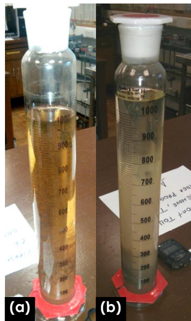
Figure 3-22: The sedimentation test after 8 days (a) the British soil (b) the Sudanese soil
