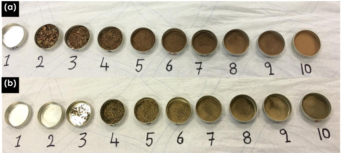
Figure 3-13: Wet sieve results for (a) the British soil (b) the Sudanese soil (for sieve sizes (from 1-10) refer to sieves arrangement in Figure 3-11).
