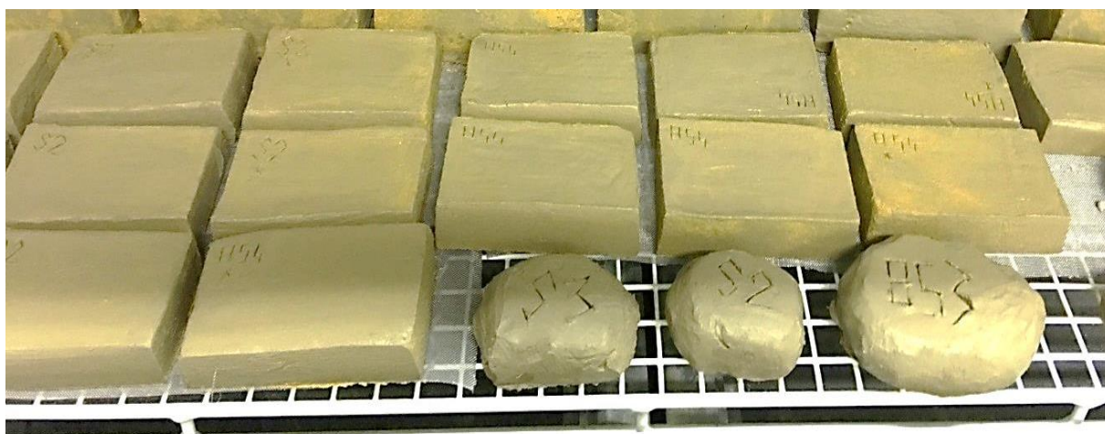
Figure 4-26: 0.5% Sudanese bovine adobe stabilised scaled bricks drying in the controlled environmental chamber
