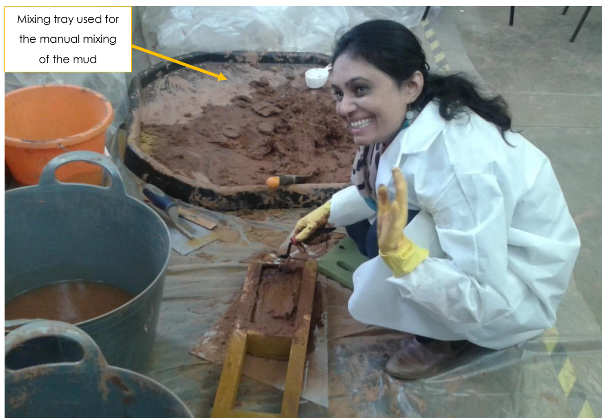
Figure 3-49: Manual mixing using mixing tray to prepare the unstabilised British adobe bricks for the preliminary experiments
