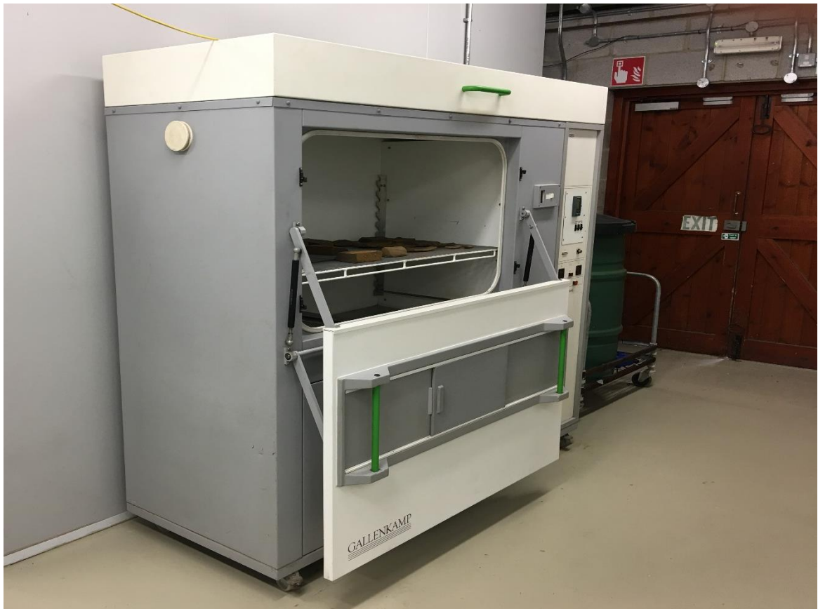
Figure 3-53: The environmental chamber used to dry the adobe bricks in this study
