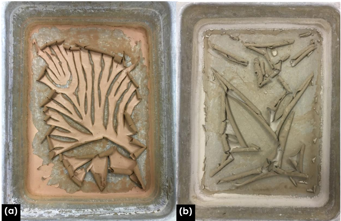
Figure 3-14: Soil particles passed 63 µm sieve after the wet sieve for (a) the British soil (b) the Sudanese soil
