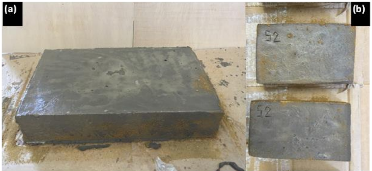
Figure 4-31: 5% Bovine stabilised Sudanese adobe bricks, (a) Full-size brick before cutting into scaled bricks, (b) Scaled bricks produced from cutting the full-size brick, this photo of the scaled bricks was taken just after the bricks finished the 16 hours of the initial drying in the laboratory environment
