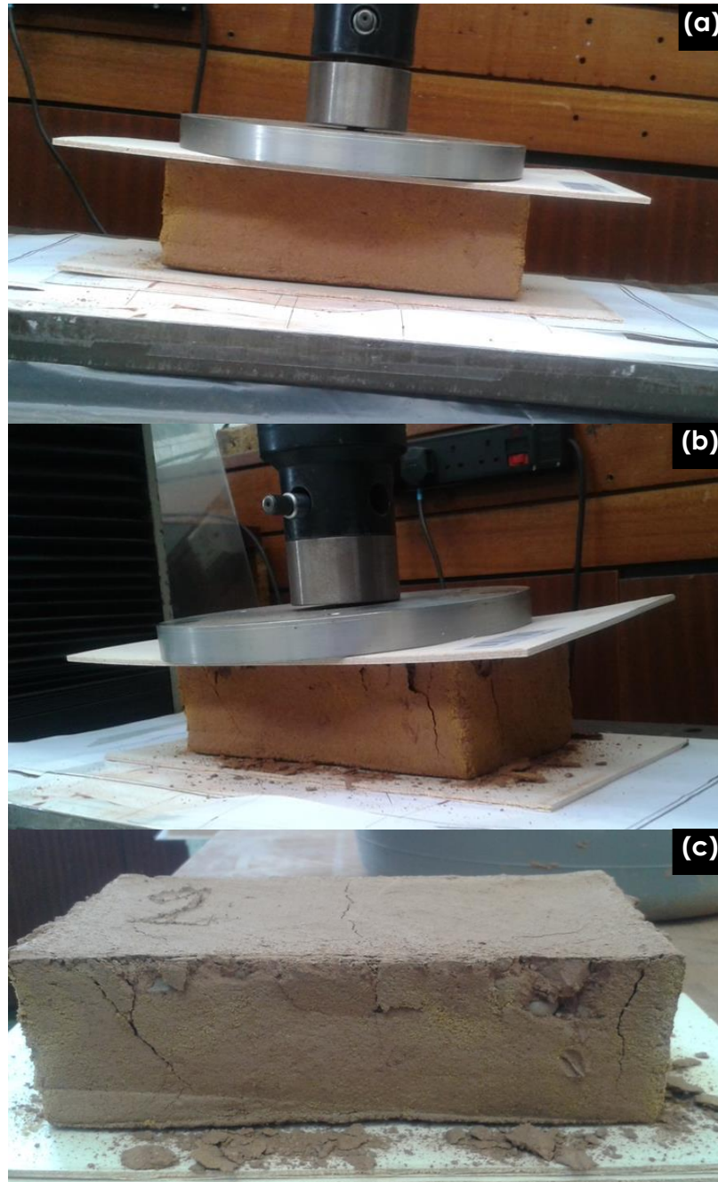
Figure 3-41: The adobe brick under the compression load using an Instron 4206 machine, (a) the setting of the brick sandwiched between two plywood pieces, (b) the adobe brick during the compressive strength test, (c) the brick after the end of the compressive strength test showing the mode of failure.
