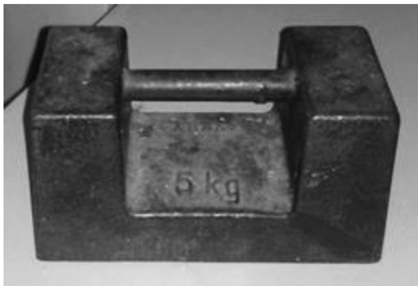
Figure 4-2: The 5 kg metal weight used when preparing the adobe full-size bricks
