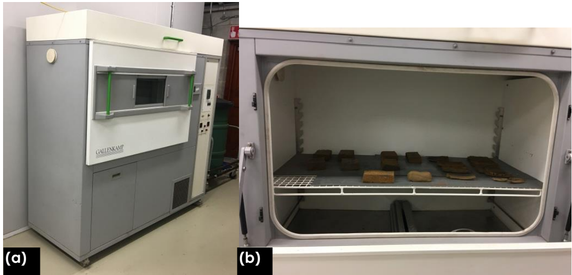
Figure 4-5: The controlled environmental chamber where all the bricks drying process in this study was taken place. The chamber was temperature and humidity controlled. (a) The chamber from the outside. (b) The chamber from the inside
