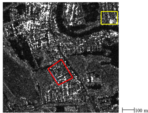
Fig. 14 CSK subimage ( 1 \times 1 km) of Thames flood in Staines, West London (pixel intensities are DN backscatter values, dark areas are water). Red outline shows the area covered by the aerial photo of Fig. 13. Yellow rectangle is high urban area.
