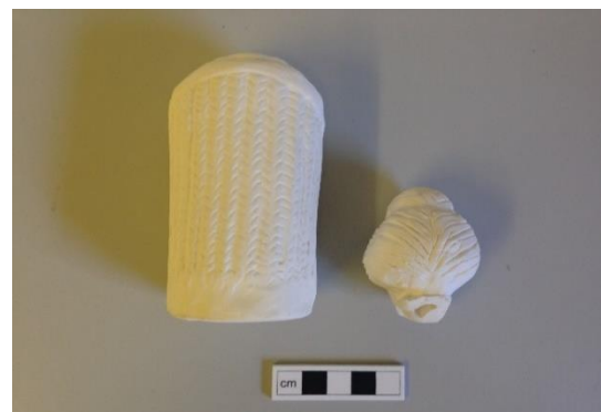
Fig. A.7. 4. Dea Nutrix figurine toppled off a ledge from standing onto a flat brick/tile surface from 50cm.
