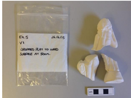
Fig. A.7. 2. Venus figurine dropped flat onto flat brick/tile surface from 50cm.
