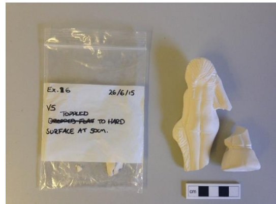
Fig. A.7. 3. Venus figurine toppled off a ledge from standing onto flat brick/tile surface from 50cm.
