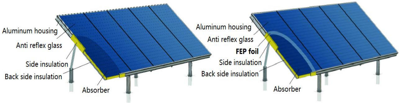
Figure 11 Typical large area solar collector without/with FEP foils (Source: Arcon-Sunmark A/S) [66].
